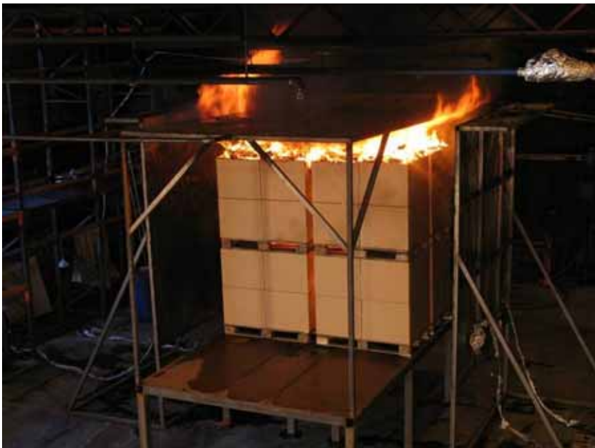
Figure A-142 Test 5S(15): Photo taken 01:00 [min:sec] after fire ignition.
