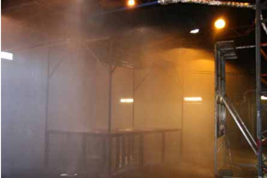
Figure A-97 Test 1S(15): The water sprays from the nozzles prior the test.
