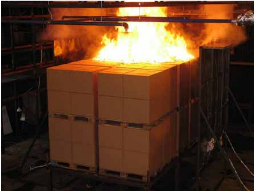
Figure A-5 Test 1E(15): Photo taken 02:00 [min:sec], at the moment the water spray system was manually activated. The fire has reached a convective heat release rate of 3000 kW and a total heat release rate of approximately 5000 kW.
