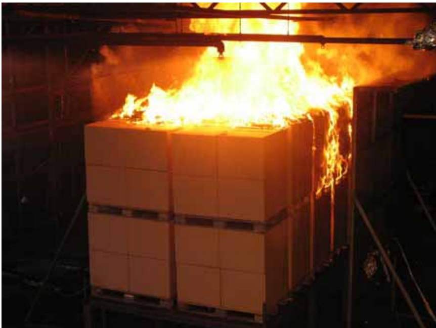
Figure 15 The fire size at the manual activation of the system during Test 8E(10), where the fire size was twice as large as in the other tests. Time 02:33 [min:sec] after fire ignition.
