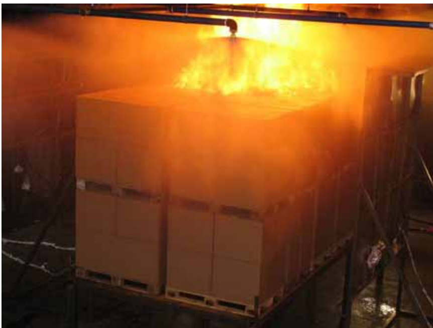
Figure A-26 Test 3E(10): Photo taken at the moment the water spray system was manually activated, 02:00 [min:sec] after fire ignition.
