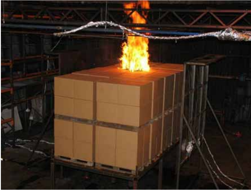
Figure A-61 Test 6E(HP-4.6): Photo taken 30 seconds after fire ignition.
