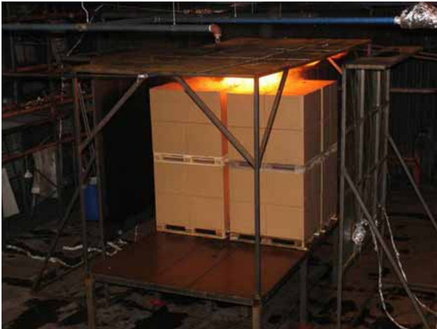
Figure A-98 Test 1S(15): Photo taken 30 seconds after fire ignition.
