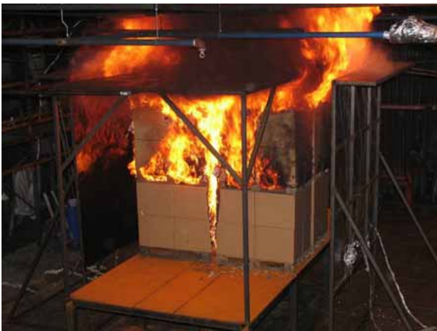
Figure A-110 Test 2S(10): Photo taken at 02:00 [min:sec] after fire ignition.
