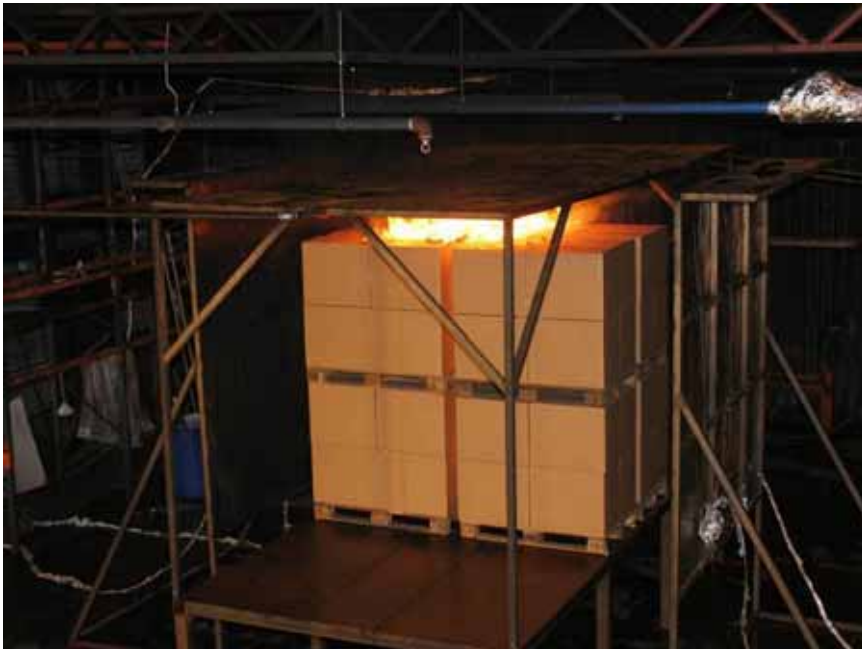
Figure A-119 Test 3S(10): Photo taken 30 seconds after fire ignition.
