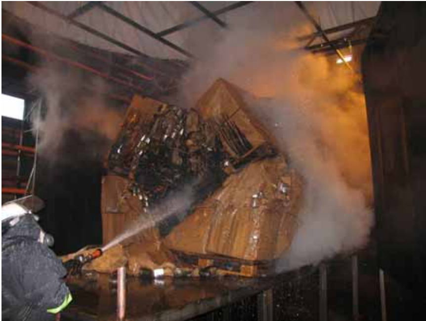
Figure A-9 Test 1E(15): Manual fire fighting of the remaining fire after the test. Note that the outer stacks of commodity have been removed in order to increase the access to the remaining (very small) fire.
