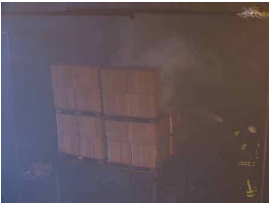
Figure A-94 Test 8E(10): Photo taken 30:15 [min:sec] after fire ignition. The water spray system has been shut off and manual fire fighting of the remaining (small) fire has started.
