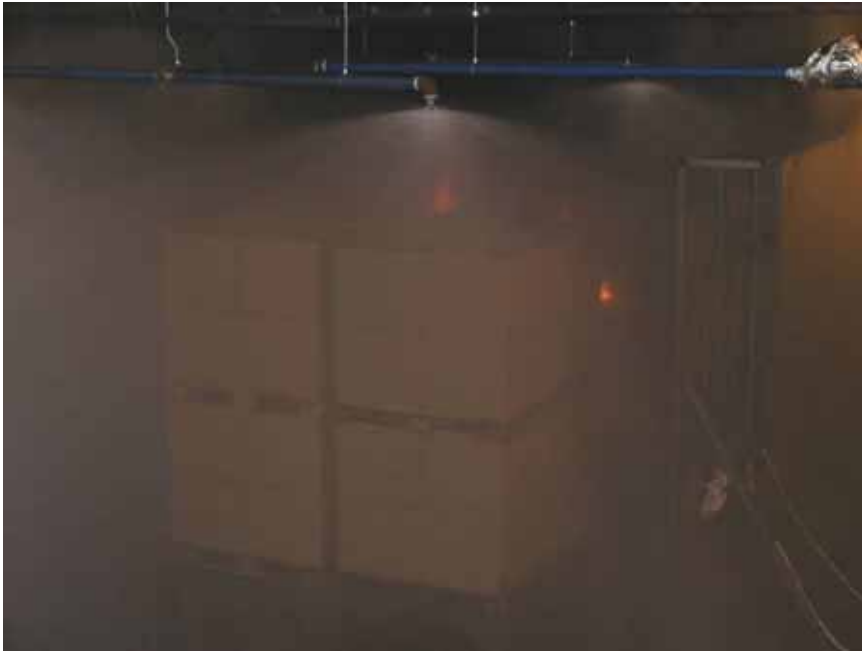
Figure A-7 Test 1E(15): Photo taken 03:00 [min:sec] after fire ignition. The fire is suppressed and only small flames are visible at the longitudinal and vertical flue spaces.
