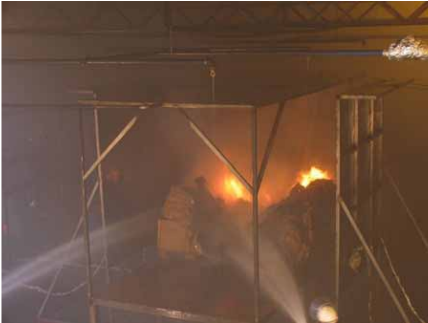
Figure A-126 Test 3S(10): Photo taken at 30:15 [min:sec] after fire ignition. The water spray system has been shut off and manual fire fighting has started.
