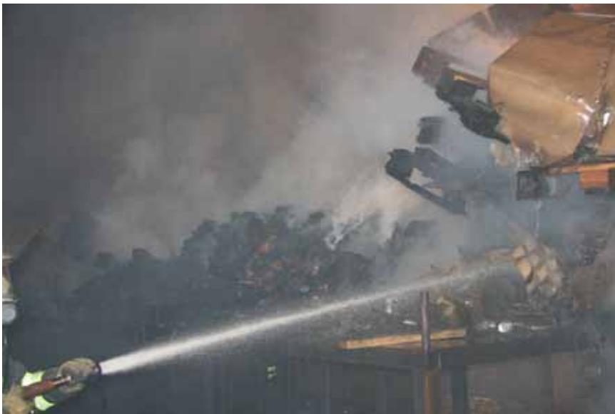
Figure A-79 Test 7E(HP-5.8): The fire damages, as seen from the left hand side, during the removal of the fire damaged pallet loads of commodity at the back end.
