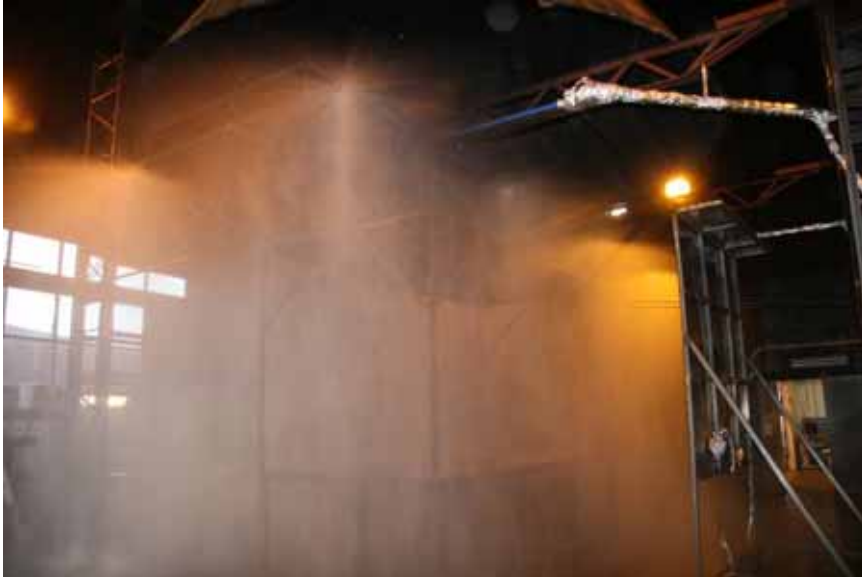
Figure A-118 Test 3S(10): The water spray prior to the test.
