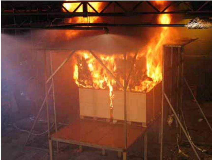
Figure A-145 Test 5S(15): Photo taken 02:13 [min:sec] after fire ignition, at the moment the water spray system was manually activated.
