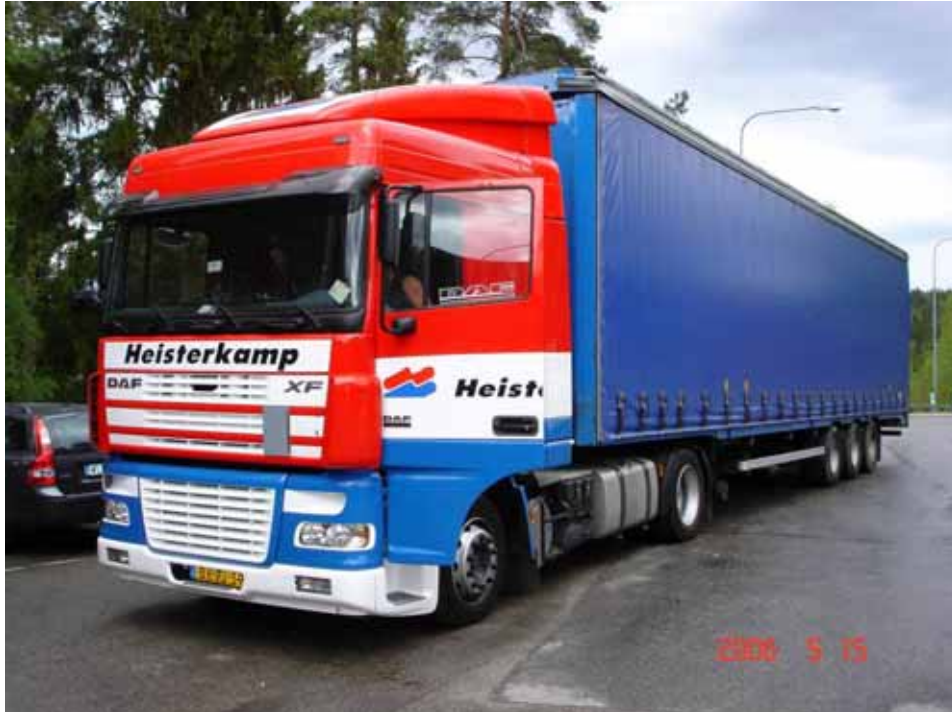
Figure 2 A common type freight truck used throughout Europe, where the trailer is covered by a tarpaulin, both on the sides (“curtain sides”) and over the top.
