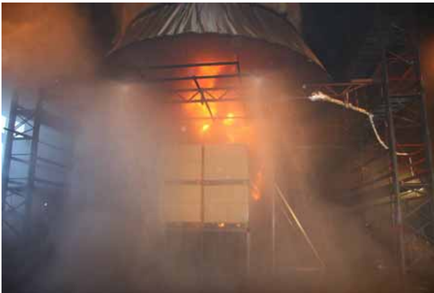
Figure A- 88 Test 8E(10): Photo taken 02:33 [min:sec] after fire ignition, at the manual activation of the water spray system as seen from floor level.
