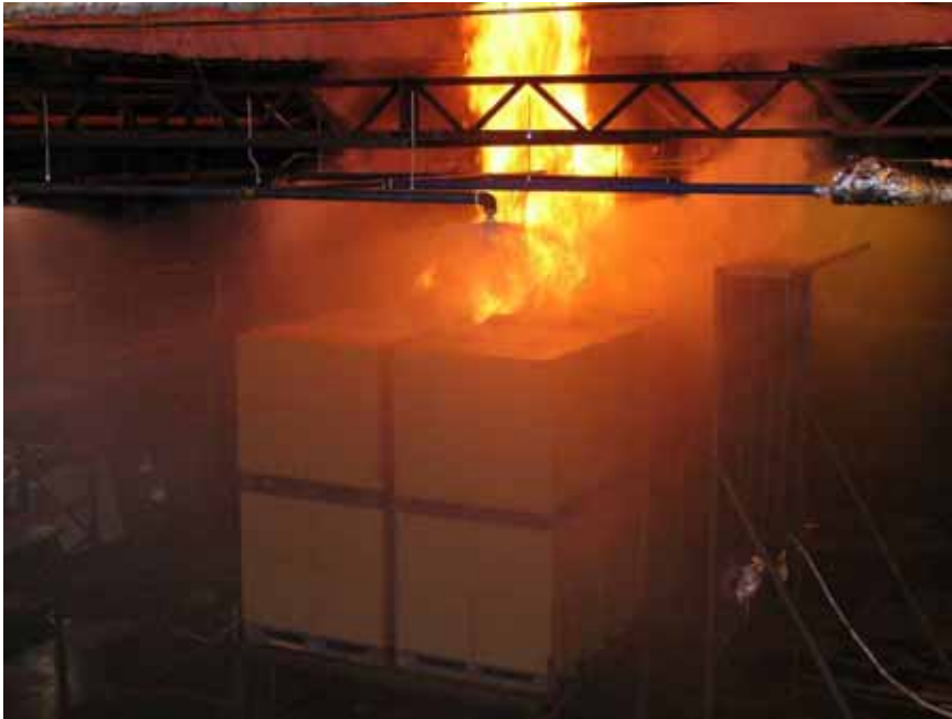
Figure A-15 Test 2E(10): Photo taken at 02:10 [min:sec], moments after the water spray system was manually activated.
