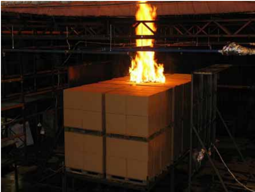
Figure A-12 Test 2E(10): Photo taken 01:00 [min:sec] after fire ignition.
