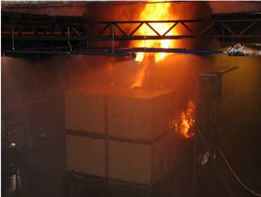
Figure A-17 Test 2E(10): Photo taken 02:30 [min:sec] after fire ignition. The fire size is controlled and flames are concentrated to the longitudinal flue space and the horizontal area between the pallet loads forming the central stack.
