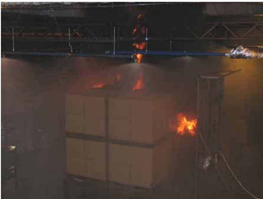
Figure A-18 Test 2E(10): Photo taken 03:00 [min:sec] after fire ignition. The fire size is controlled and flames are concentrated to the longitudinal flue space and the horizontal area between the pallet loads forming the central stack.
