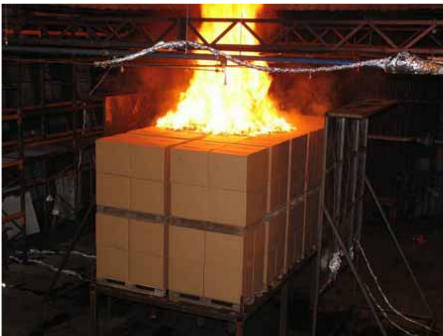
Figure A-64 Test 6E(HP-4.6): Photo at about 01:40 [min:sec] after fire ignition, a few seconds prior to the manual activation of the high-pressure water mist system.
