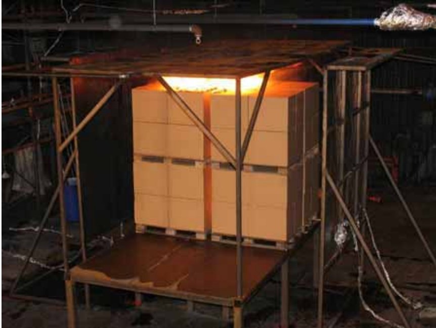
Figure A-129 Test 4S(5): Photo taken 30 seconds after fire ignition.
