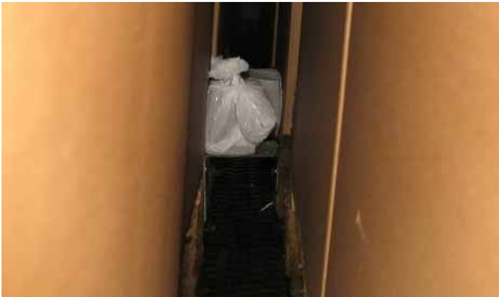
Figure 13 The standardised igniters that consisted of a cube from pieces of insulating fibre board soaked with heptane and wrapped in a polyethylene plastic foil bag.
