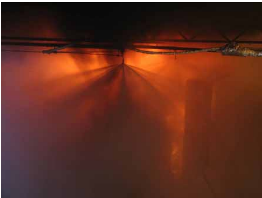
Figure A-57 Test 5E(HP-3,75): Photo taken 05:00 [min:sec] after fire ignition. The fire is not controlled by the system.
