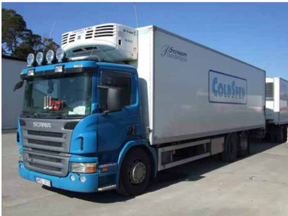
Figure 3 A common type freight truck used for temperature controlled (freezer or refrigeration) transportation of for example food products.
