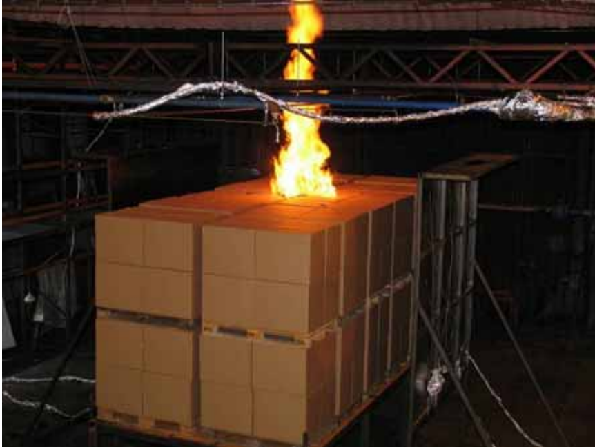
Figure A-52 Test 5E(HP-3,75): Photo taken 30 seconds after fire ignition.
