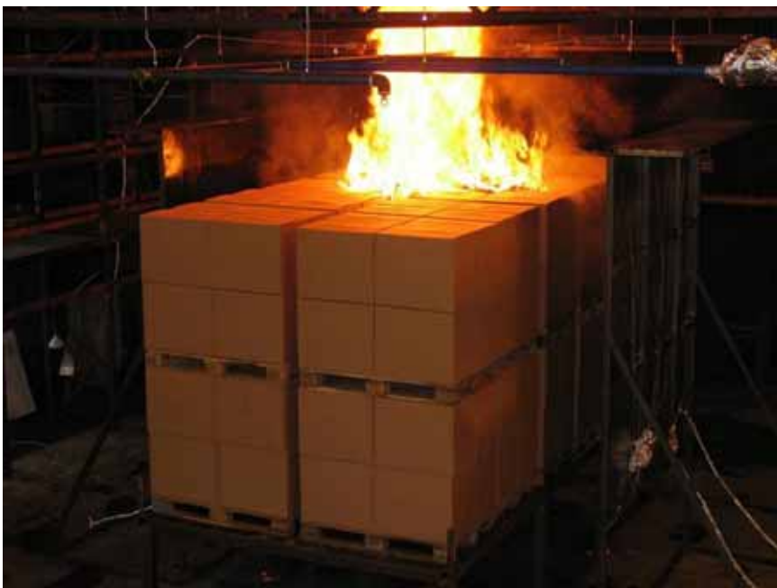
Figure A-4 Test 1E(15): Photo taken 01:30 [min:sec] after fire ignition. The top surface of the commodity has started to become involved in the fire.
