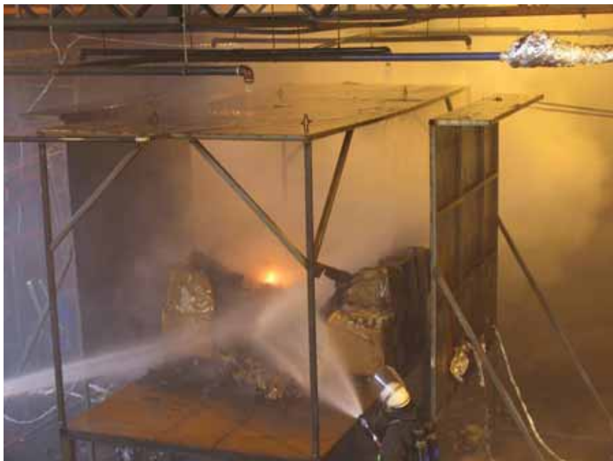
Figure A-115 Test 2S(10): Photo taken at 30:15 [min:sec] after fire ignition. The water spray system has been shut off and manual fire fighting has started.
