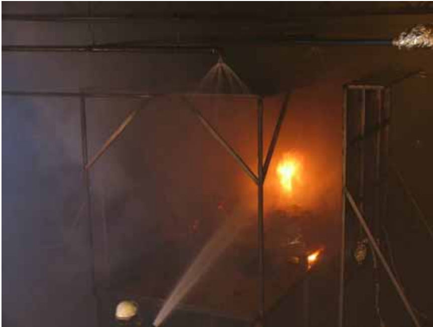
Figure A-149 Test 5S(15): Photo taken 30:15 [min:sec] after fire ignition. The water spray system has been shut off and manual fire fighting has started.
