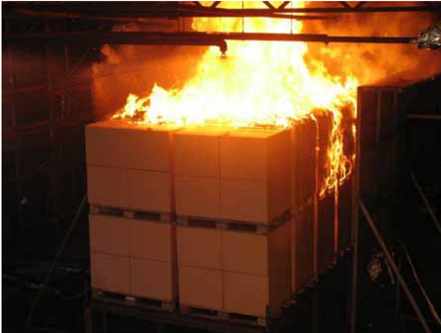
Figure A-87 Test 8E(10): Photo taken 02:33 [min:sec] after fire ignition, at the manual activation of the water spray system.
