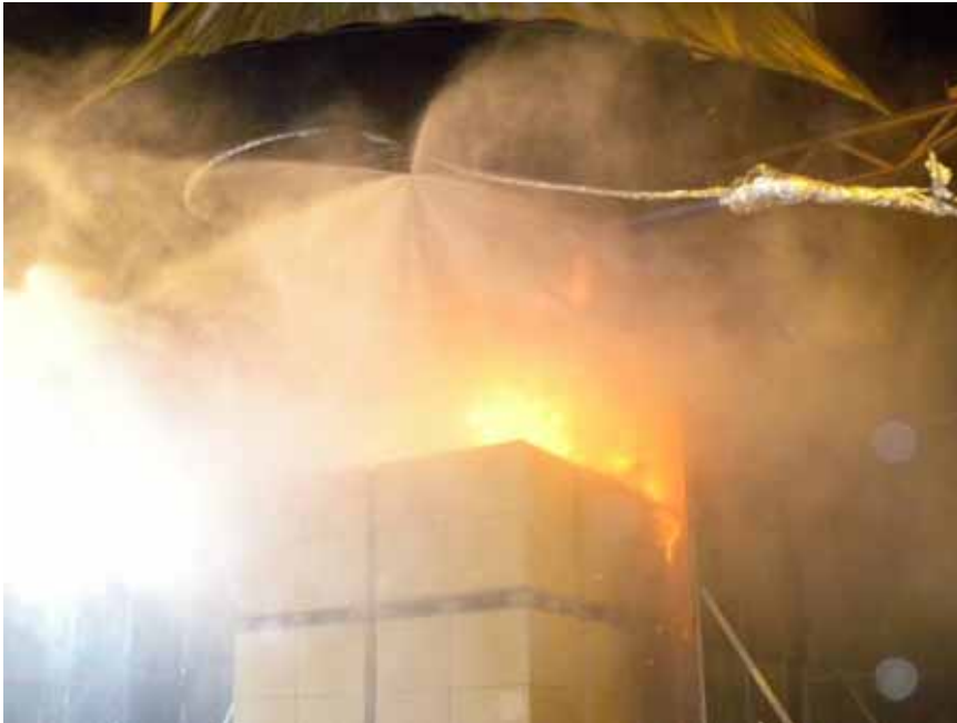
Figure A-74 Test 7E(HP-5.8): Photo taken at approximately 02:06 [min:sec] after fire ignition, soon after the manual activation of the high-pressure water mist system.
