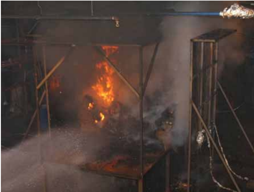
Figure A-139 Test 4S(5): Photo taken 30:15 [min:sec] after fire ignition. The water spray system has been shut off and manual fire fighting has started.
