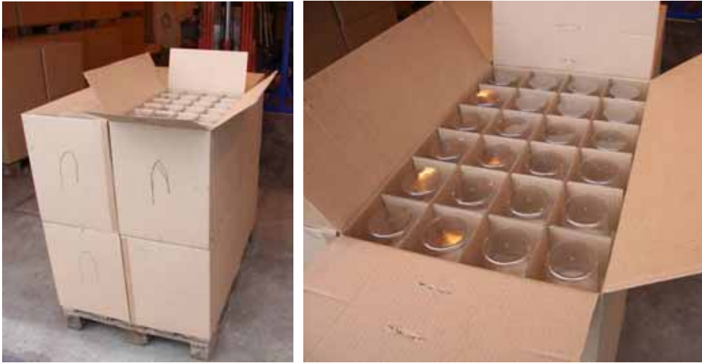
Figure 6 One pallet load of the EUR Std plastic commodity (left) with a close-up photo of the arrangement of the plastic cups in the individual cartons (right).
