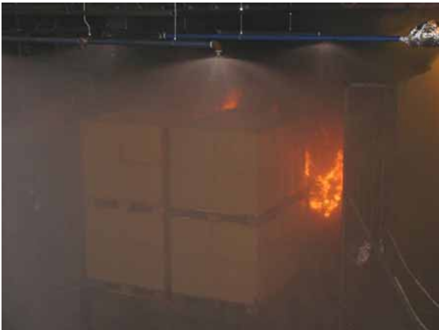
Figure A-6 Test 1E(15): Photo taken 02:30 [min:sec] after fire ignition. The fire is suppressed and flames are concentrated to the longitudinal flue space and the horizontal area between the pallet loads forming the central stack.
