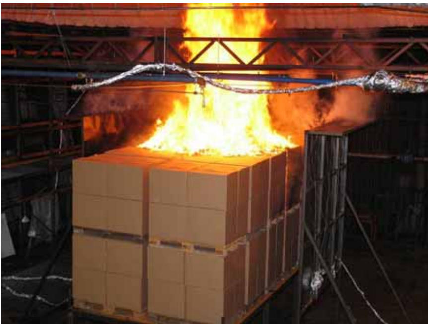
Figure A-55 Test 5E(HP-3,75): Photo taken at the moment the high-pressure water mist system was manually activated, 01:58 [min:sec] after fire ignition.
