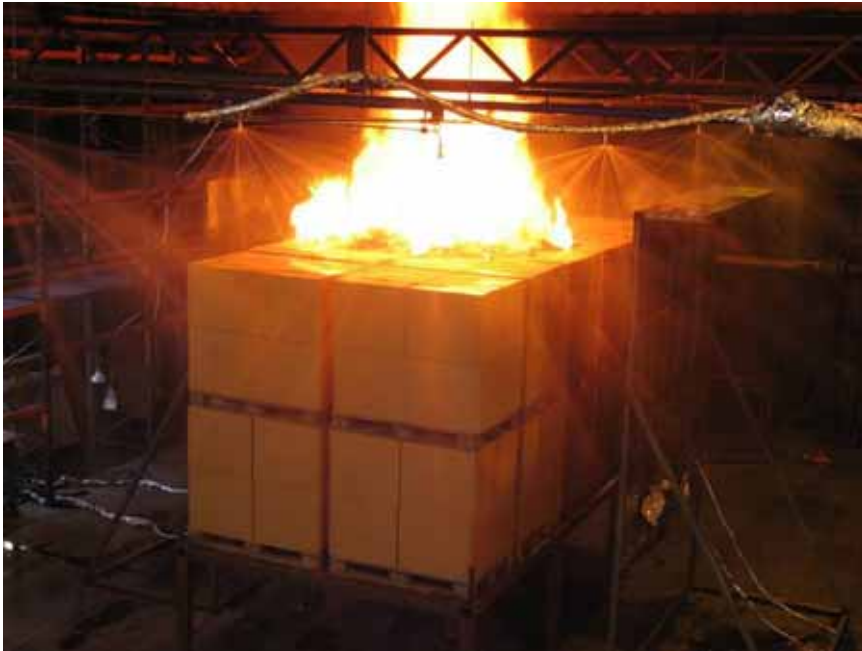
Figure A-65 Test 6E(HP-4.6): Photo at 01:45 [min:sec] after fire ignition, at the manual activation of the high-pressure water mist system.
