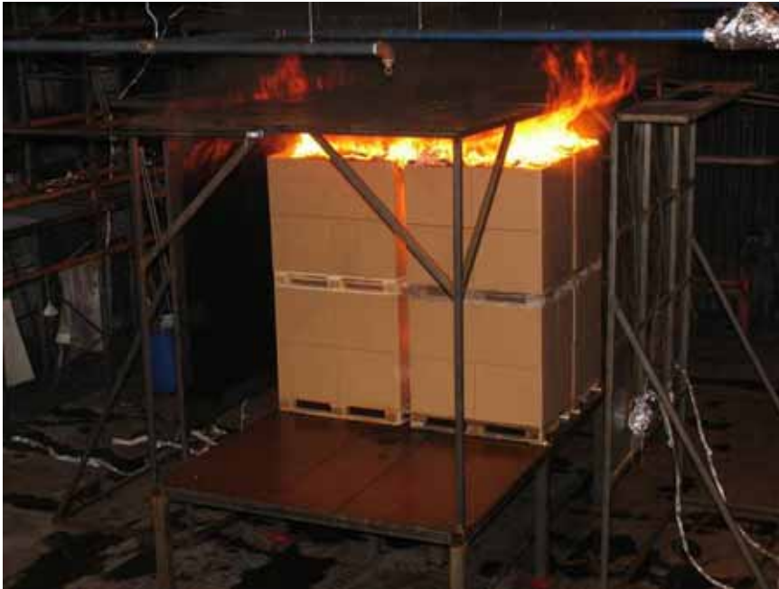
Figure A-99 Test 1S(15): Photo taken 01:00 [min:sec] after fire ignition.
