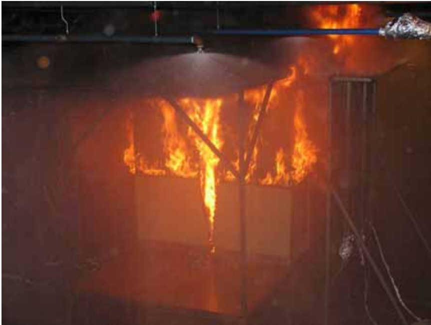
Figure A-111 Test 2S(10): Photo taken at 02:12 [min:sec] after fire ignition, at the moment the water spray system was manually activated.
