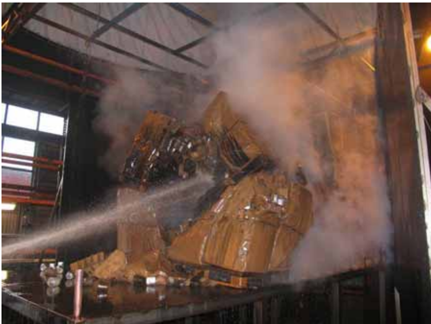
Figure A-10 Test 1E(15): Manual fire fighting of the remaining fire after the test. Note that the outer stacks of commodity have been removed in order to increase the access to the remaining (very small) fire.
