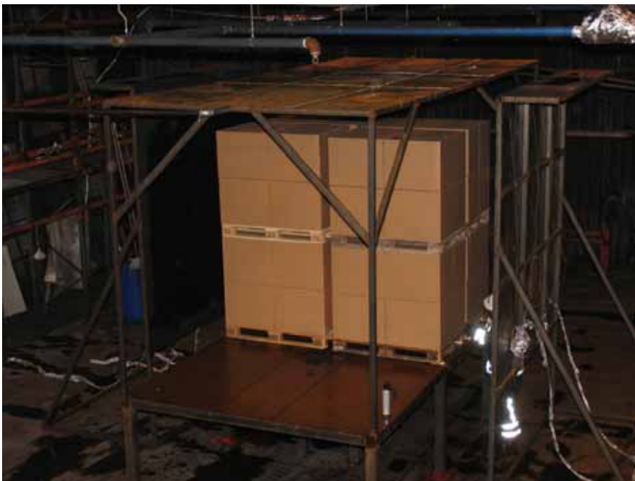
Figure 5 The trailer mock-up with the roof installed. Note that less amount of commodity, two instead of six rows was used for these tests.
