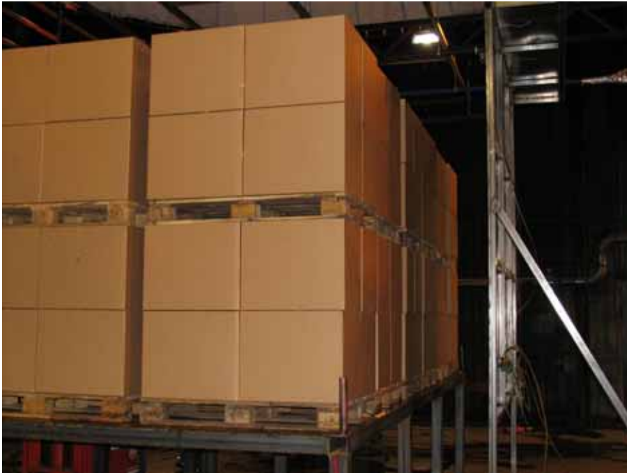
Figure 4 An illustration of the arrangement of the commodity on the trailer mock-up, showing the steel screen on the right hand long side. A similar screen was positioned on the left hand side.
