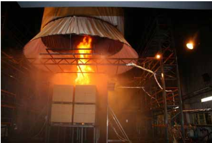
Figure A-16 Test 2E(10): The fire size at moments after the water spray system was manually activated, as seen from floor level.
