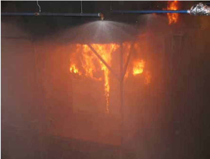
Figure A-103 Test 1S(15): Photo taken 02:45 [min:sec] after fire ignition, a few seconds after the manual activation of the system.
