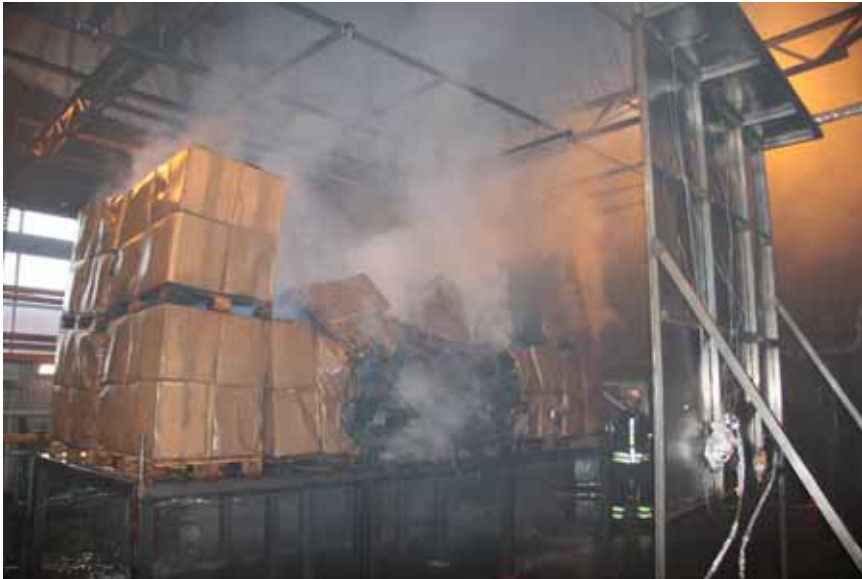
Figure A-49 Test 4E(5): Fire damages as seen from the right hand side.
