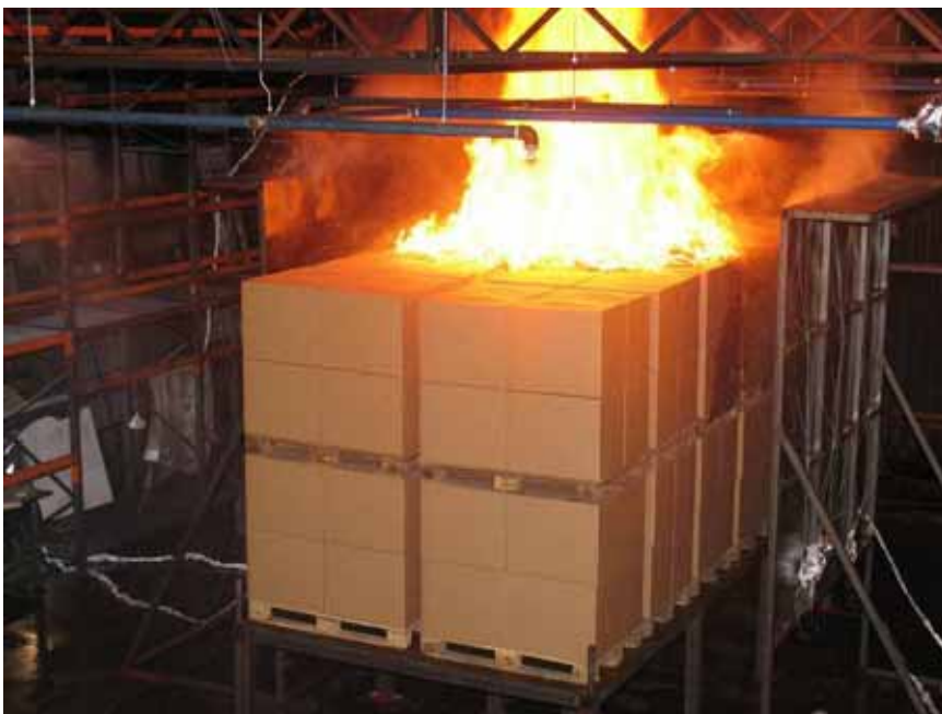
Figure A-36 Test 4E(5): Photo taken at the moment the water spray system was manually activated, 01:58 [min:sec] after fire ignition.
