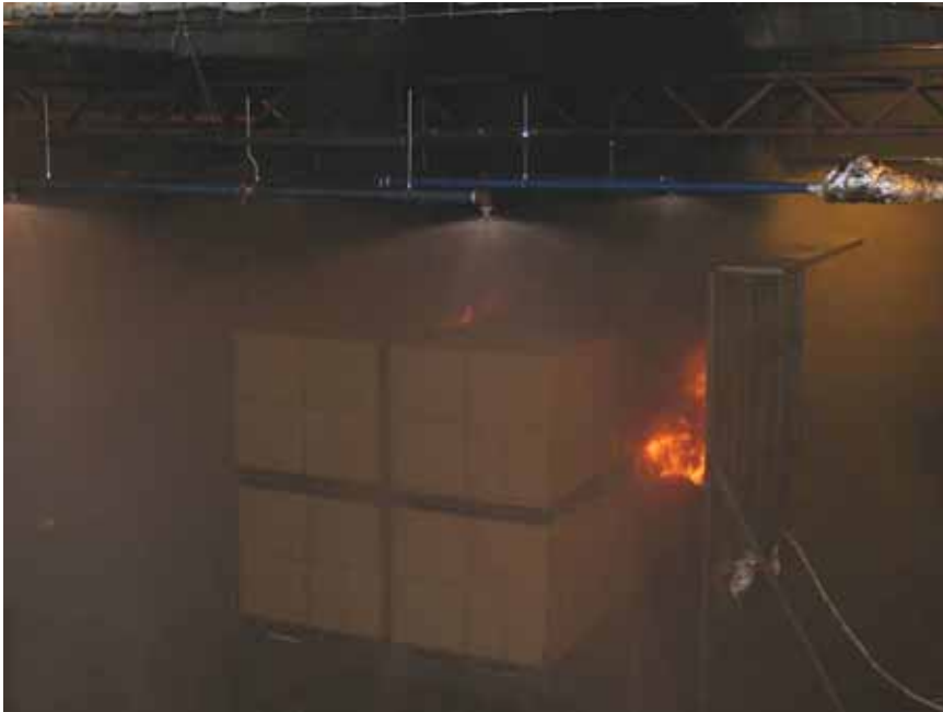
Figure A-19 Test 2E(10): Photo taken 03:30 [min:sec] after fire ignition. The fire size is controlled and flames are concentrated to the longitudinal flue space and the horizontal area between the pallet loads forming the central stack.
