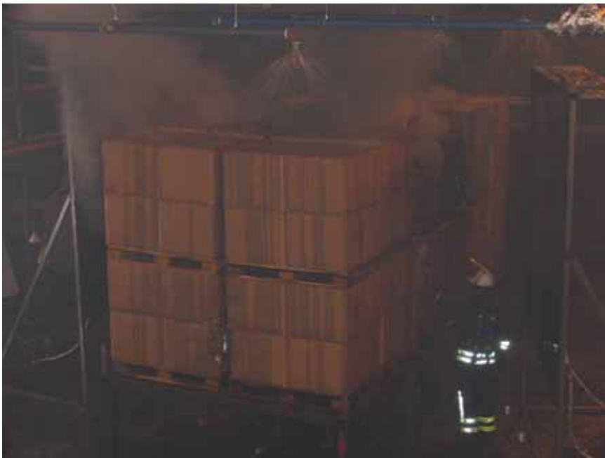
Figure A-8 Test 1E(15): The initiation of manual fire fighting 10:00 [min:sec] after fire ignition.
