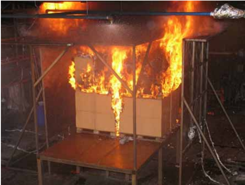
Figure A-133 Test 4S(5): Photo taken at 02:25 [min:sec] after fire ignition, at the moment the water spray system was manually activated.
