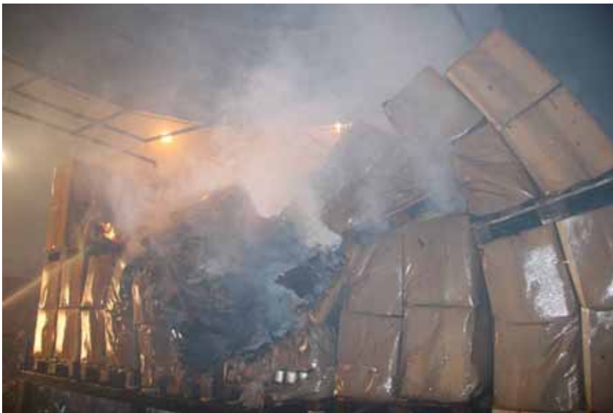
Figure A-96 Test 8E(10): Fire damages as seen from the right hand side.
