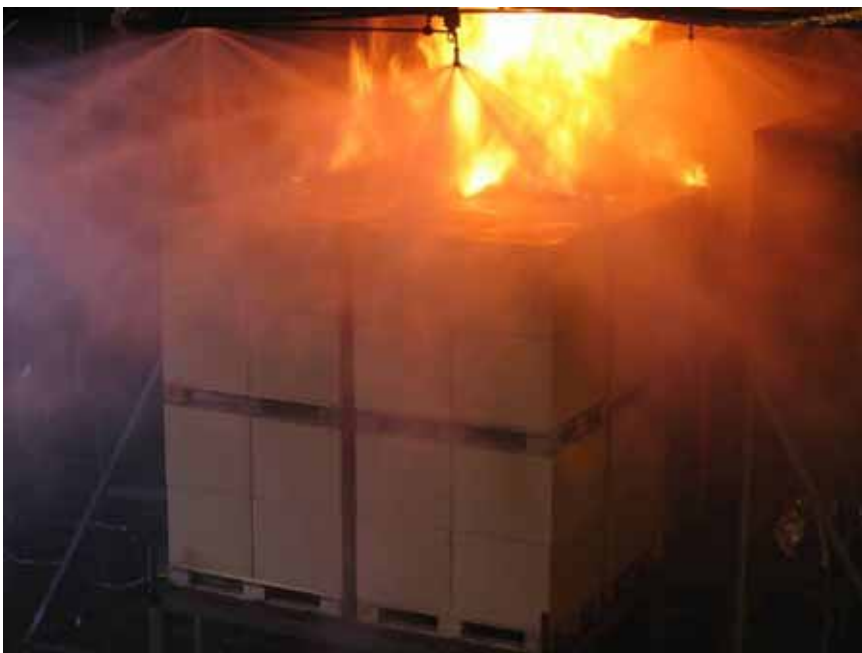
Figure A-73 Test 7E(HP-5.8): Photo taken 02:04 [min:sec] after fire ignition, at the manual activation of the high-pressure water mist system.
