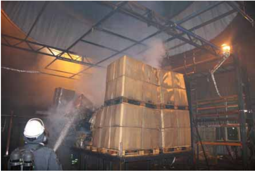
Figure A-51 Test 4E(5): Fire damages as seen from the front short side.
