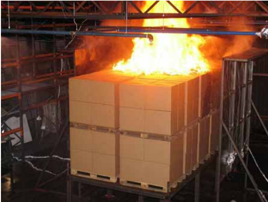
Figure 14 The fire size at the manual activation of the system for the tests without the roof of the trailer mock-up, here exemplified with Test 4E(5). Time 01:58 [min:sec] after fire ignition.
