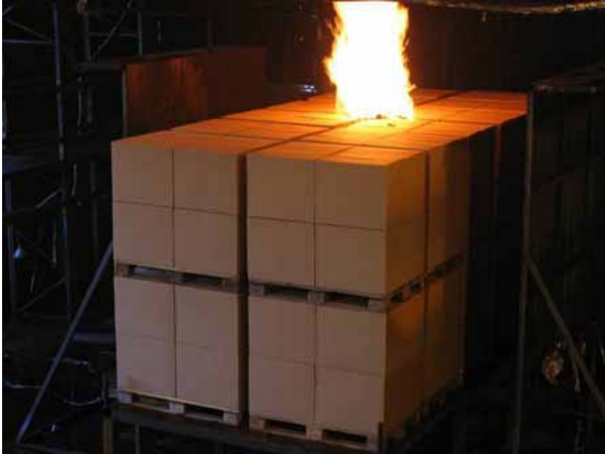
Figure A-70 Test 7E(HP-5.8): Photo taken 30 seconds after fire ignition.
