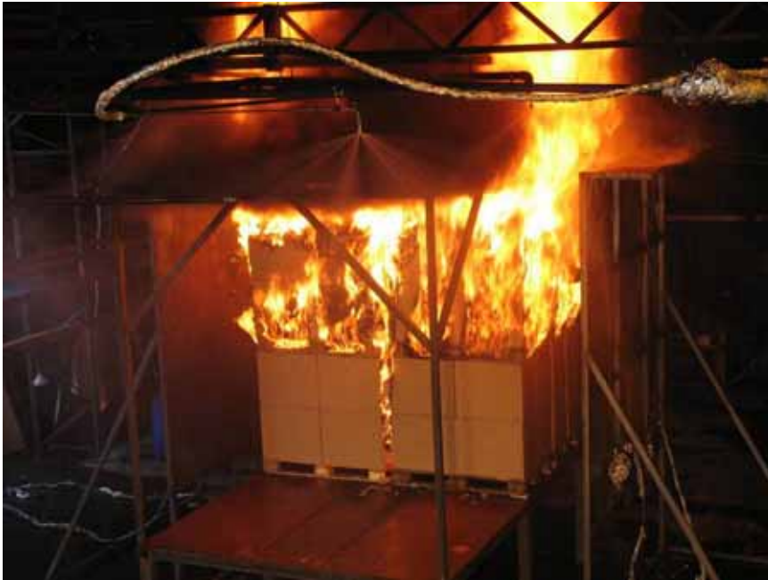
Figure A-156 Test 6S(HP-5.8): Photo taken 02:35 [min:sec] after fire ignition, at the moment the high-pressure water mist system was manually activated.
