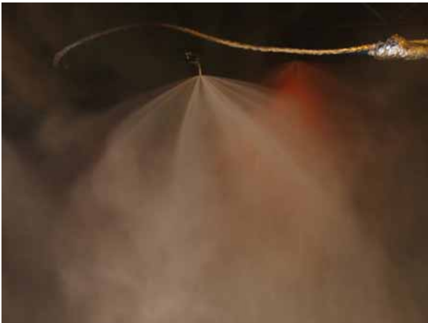
Figure A-157 Test 6S(HP-5.8): Photo taken 03:00 [min:sec] after fire ignition. The visibility is obscured by the water spray.
