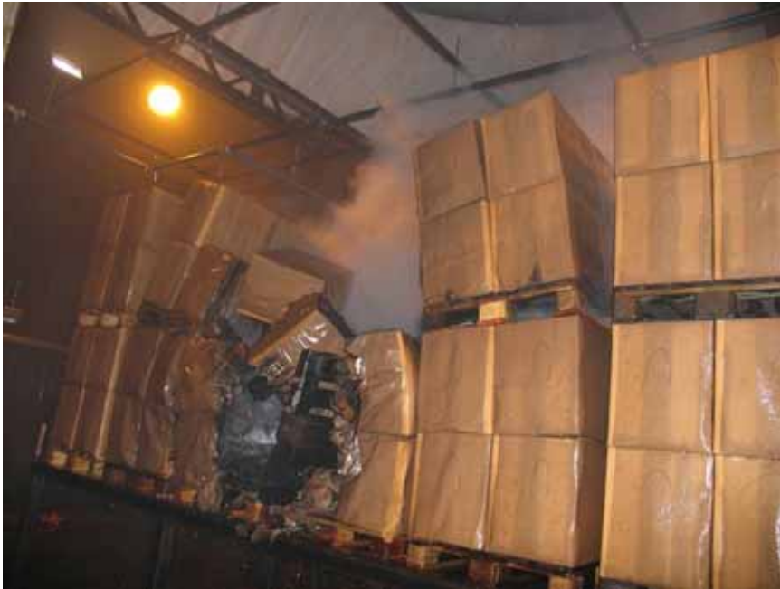
Figure A-21 Test 2E(10): Fire damages, as seen from the left hand side.
