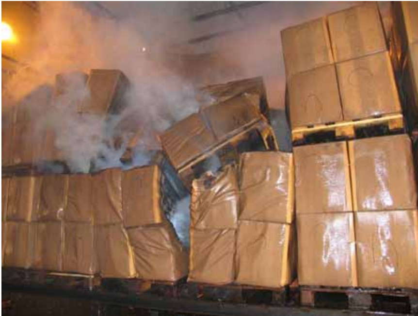
Figure A-31 Test 3E(10): Fire damages as seen from the left hand side.
