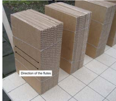
Figure 8: Cassettes of corrugated cardboard fixed with wire.
