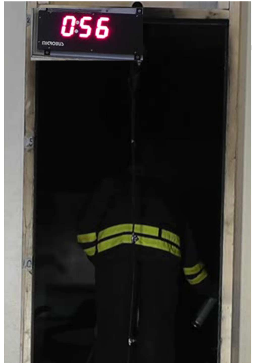
Test 18: Drencher + WMS [ 5 + 6 litres/m 2 /minute]
