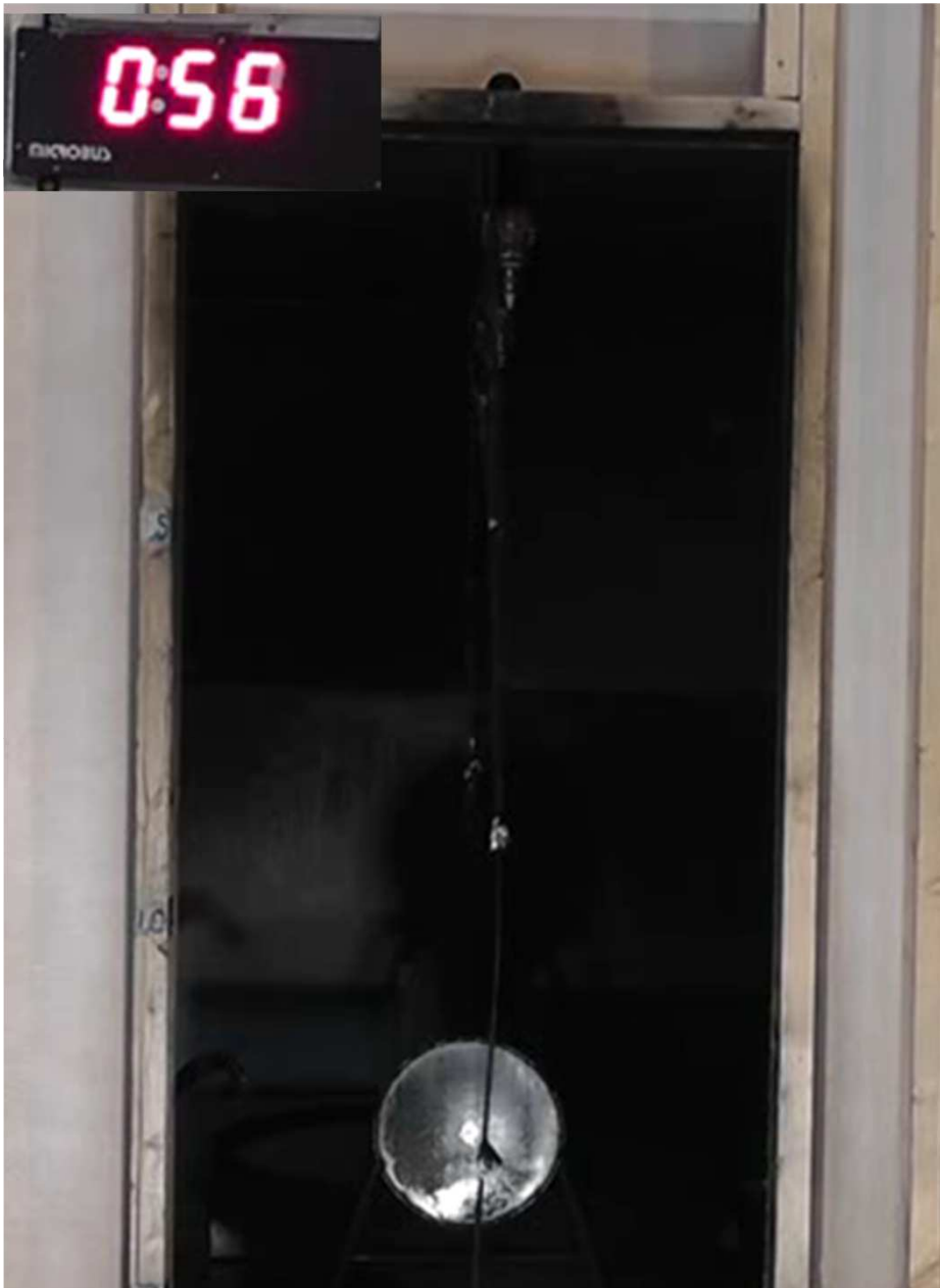
Test 16: Drencher Fuel pan #1 [32 litres/m 2 /min.]
