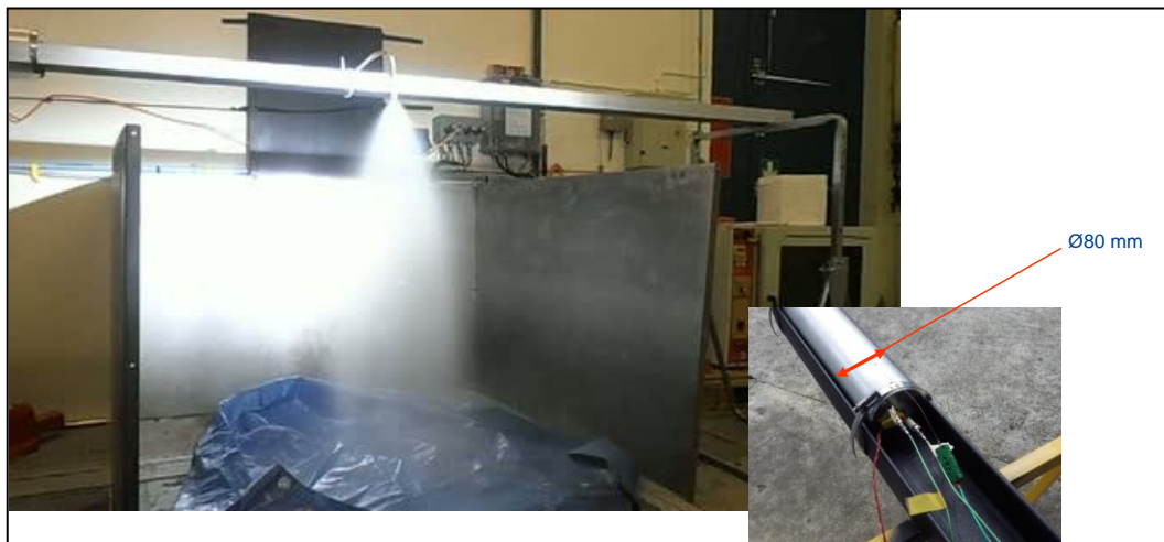
Figure 13a - Spraying test of Typhoon™ Ø80 mm - 1 l capacity with liquid agent
