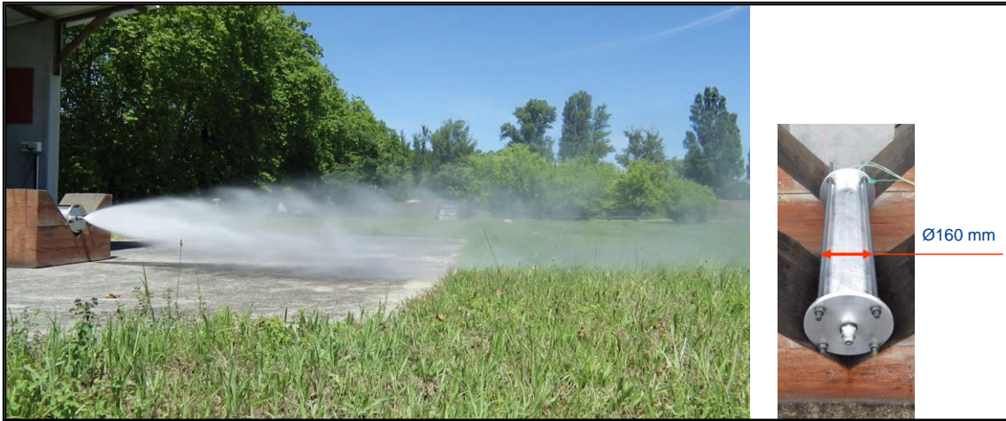
Figure 14 - Spraying test of Typhoon™ Ø160 mm - 8 l capacity with water
