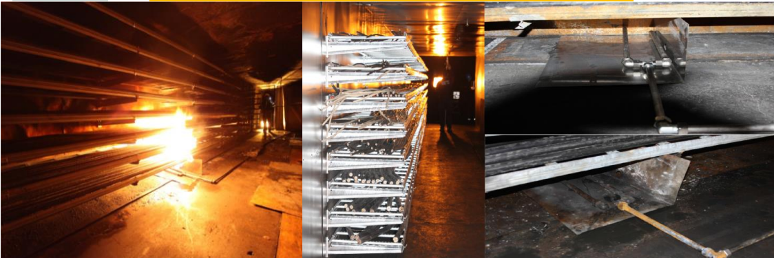
Water mist system activated during about 960 s
