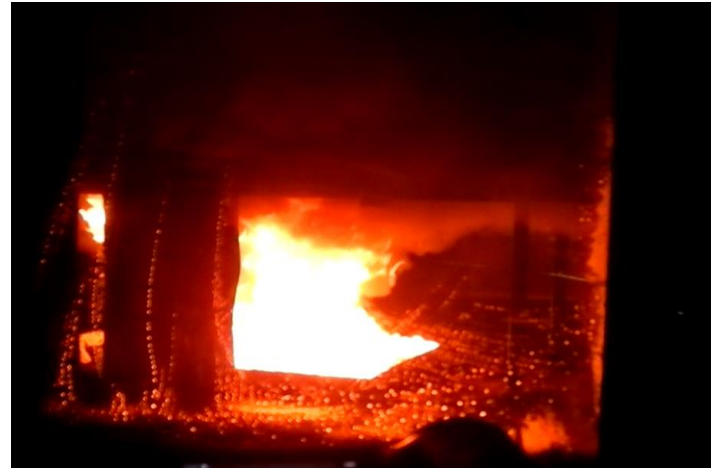
Fire tests were based on D4.3 and D4.4 in FM5560 Appendix D.
