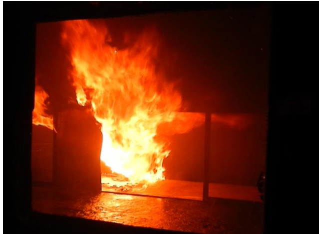
Fire tests were based on D4.3 and D4.4 in FM5560 Appendix D.
