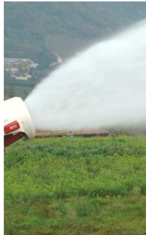
High flow mode water mist 0 to 3.500 l/min
