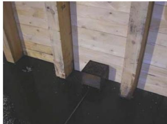
Gas burner set to generate 100kW
