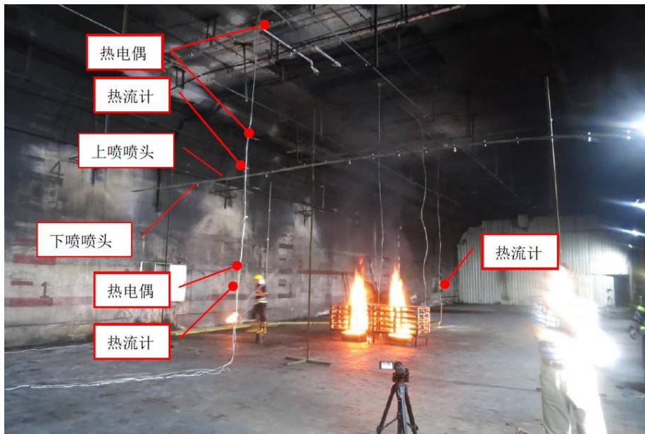
Fire load HRR 3 MW
