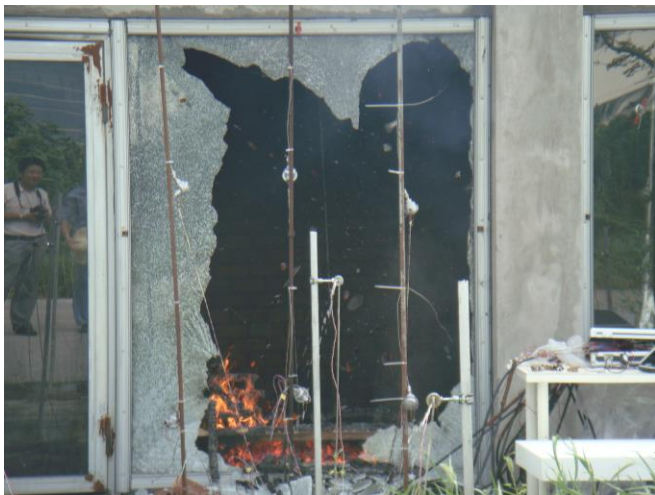
Glass break without protection by water mist
