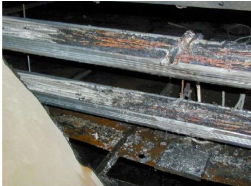
Fire damages after representative test for concealed spaces containing cables in offices (left sprinkler system and right water mist HI-FOG)
