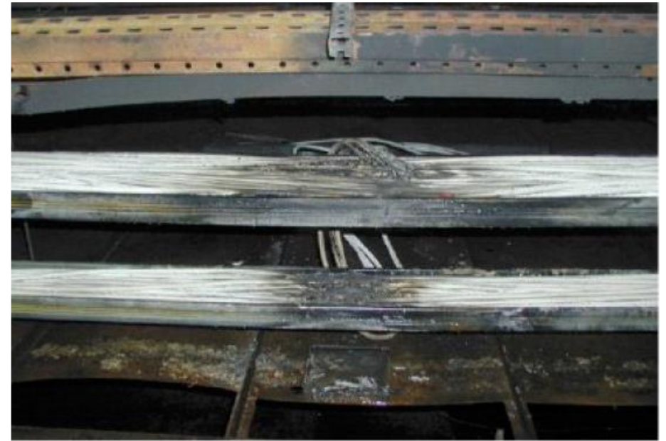
Fire damages after representative test for concealed spaces containing cables in offices (left sprinkler system and right water mist HI-FOG)
