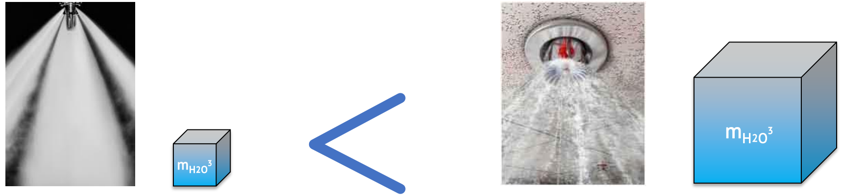
Water consumption (left water mist HI-FOG and right sprinkler system)
