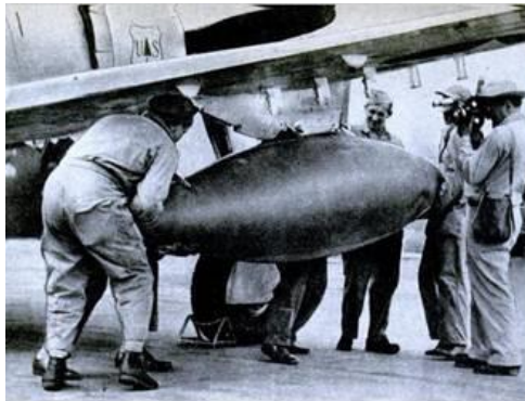
Fig. 6 Water-filled drop tank on US P-47 fighter plane
