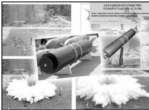
Fig. 7 Russian ASP-500 Fire-extinguishing Air System
