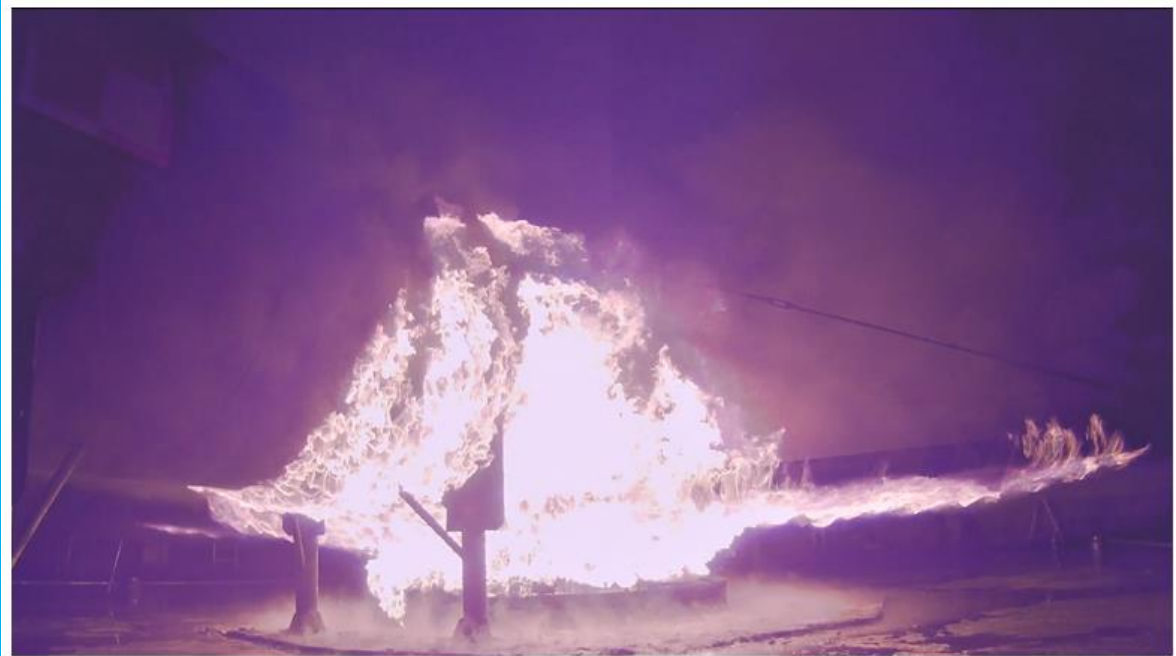
Fire developed 60seconds after ignition – pre burn time end.
