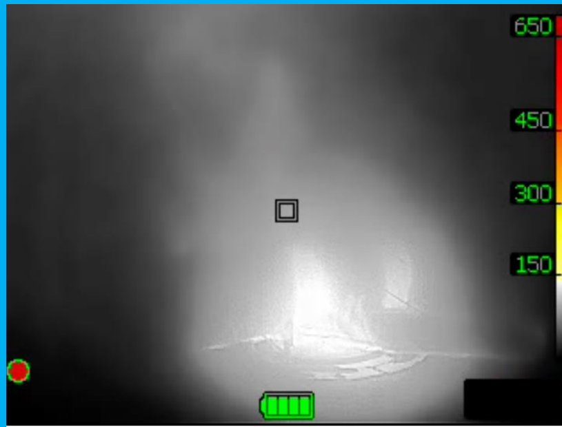
Fire in 10min after high pressure mist discharge (60 sec pre-burn + 600sec discharge) after - end of test data record - pass / fail criteria.
