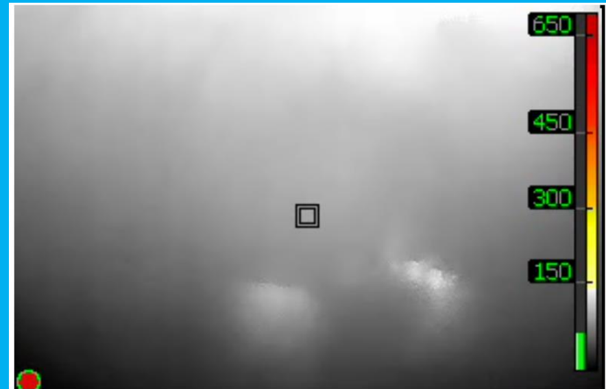
Fire in 10min after high pressure mist nozzles discharge (60 sec pre-burn + 600sec discharge) after system discharge – end of test data record - pass / fail criteria.
