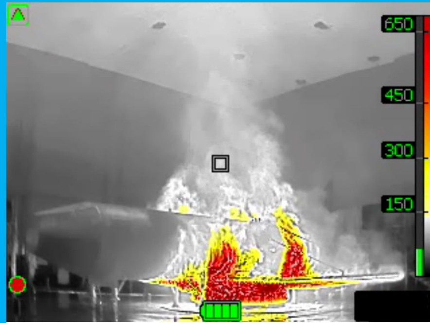
Fire developed 60 seconds after ignition – thermal view.
