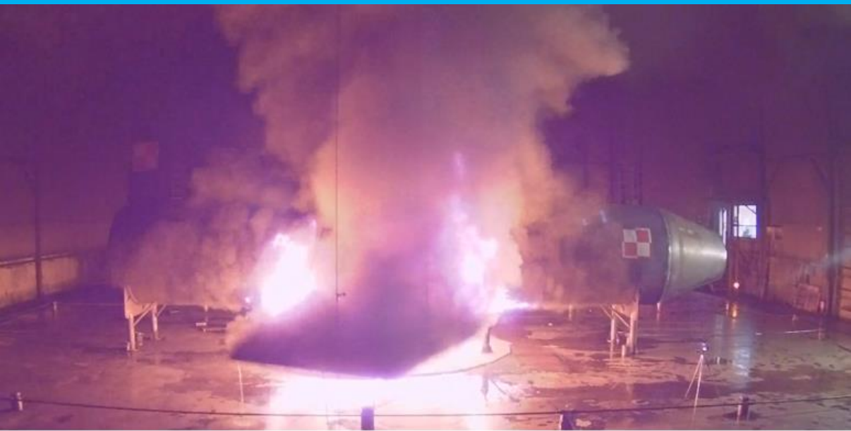
Fire developed 60seconds after ignition – pre burn time end.
