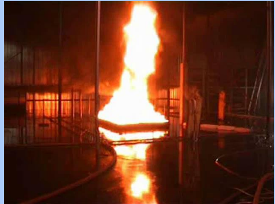
Test with 6m 2 jet fuel fire
