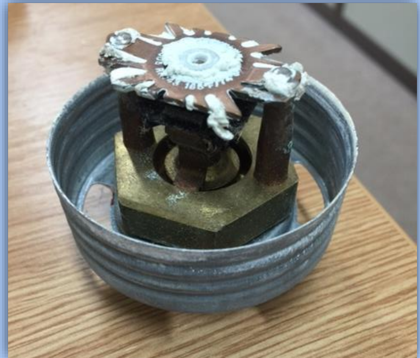
Corrosion inside sprinkler
