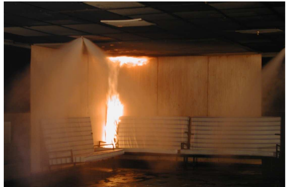
fire development in the disabled nozzle test
