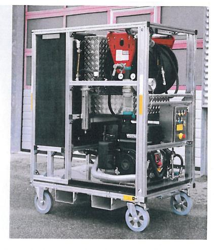
Oliver Callies explains: "This system was developed some time ago but we advance and enhance it constantly. Normally the trolleys incorporate a 300 to 450-litre tank but we have constructed a lighter and more compact 100-litre tank."
