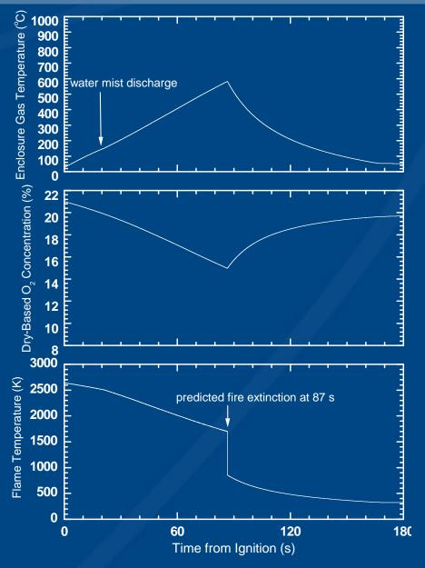
Enclosure: 7.3x7.3x5 m high Door opening: 0.9 x 2.2 m high Fuel: heptane Heat release rate: 2 MW Mist: 45 lpm Nitrogen: 0 cfm
