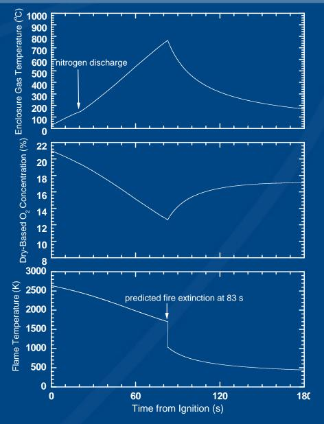
Enclosure: 7.3x7.3x5 m high Door opening: 0.9 x 2.2 m high Fuel: heptane Heat release rate: 2 MW Mist: 15.1 lpm Nitrogen: 0 cfm
