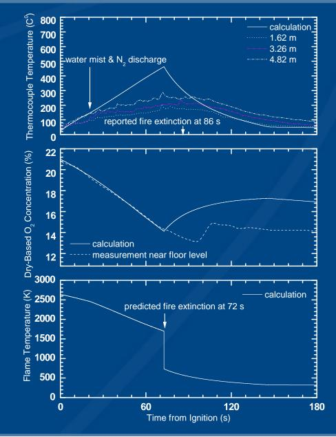
Enclosure: 7.3x7.3x5 m high Door opening: 0.9 x 2.2 m high Fuel: heptane Heat release rate: 2 MW Mist: 0 lpm Nitrogen: 600 cfm
