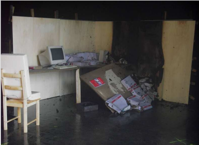
Fuel package after sprinkler fire test
