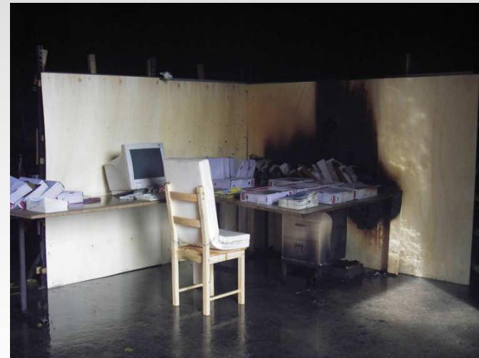
Fuel package after water mist fire test
