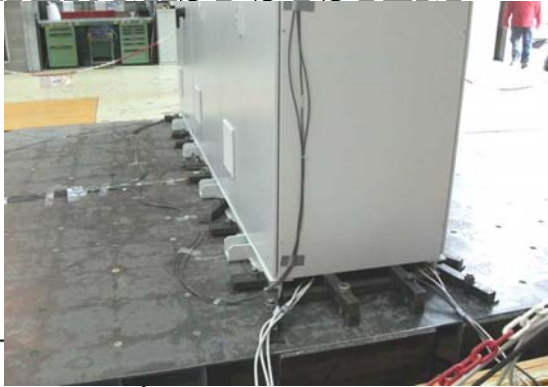
MASTER VIBRATION SYSTEM Multi Axis Shaking Table for Earthquakes Reproduction
