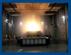
Comparable spray patterns, droplet sizes and discharge rates at the same operating pressures among different ESFR sprinklers
