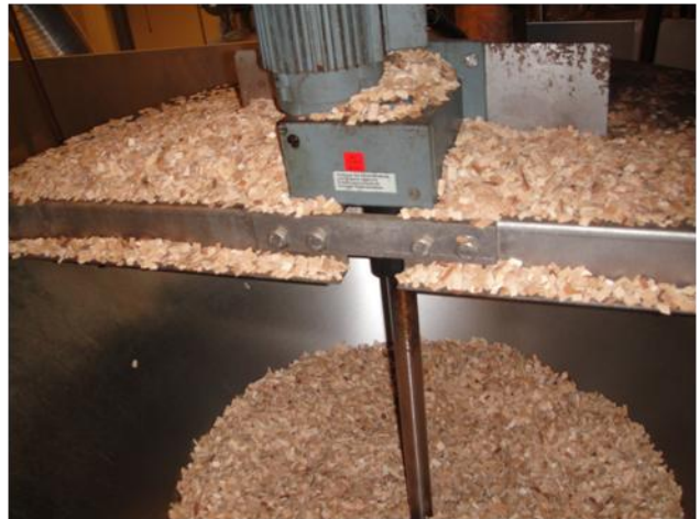
Wood Chips filled to the funnel of the smoke generator. Fully loaded approx. 50kgs of chips
