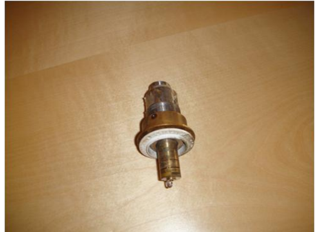
The XFLOW nozzle after release and fire, no visual damage.
