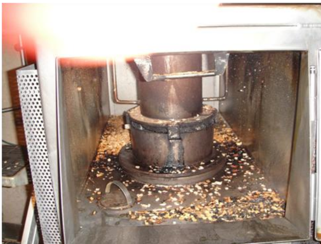
Lower part of smoke generator with the heated chamber.
