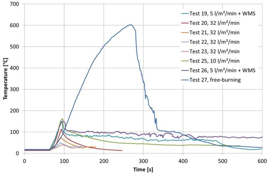
Figure 9 Dummy torpedo temperatures with fuel pan in Position 2 (beside the ordnance dummy).
