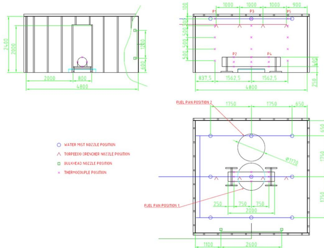
Figure 1 Test compartment
