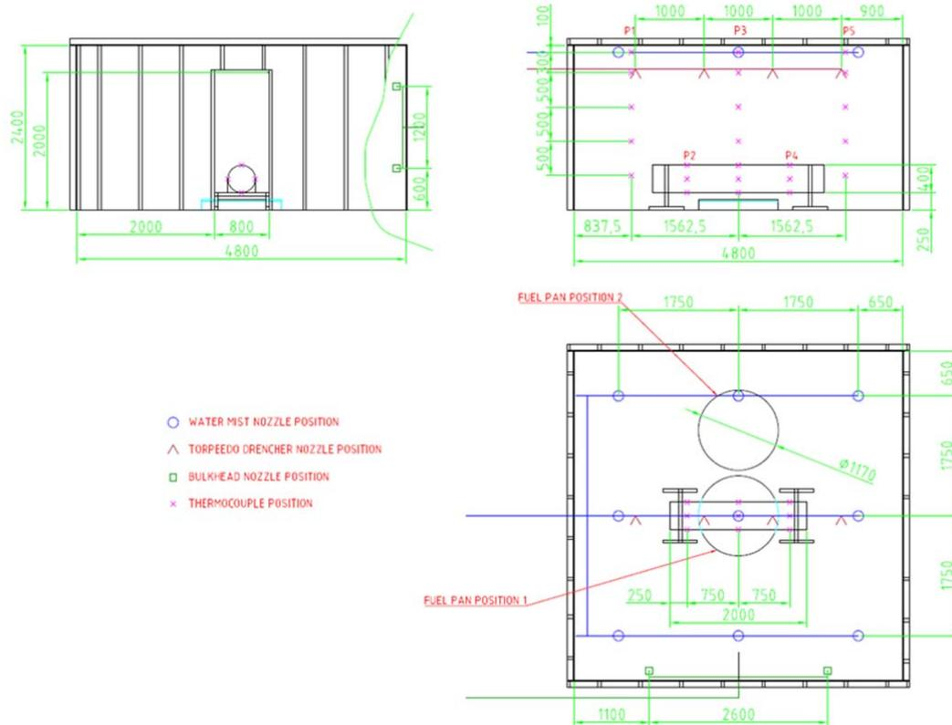
Figure 1 Test compartment
