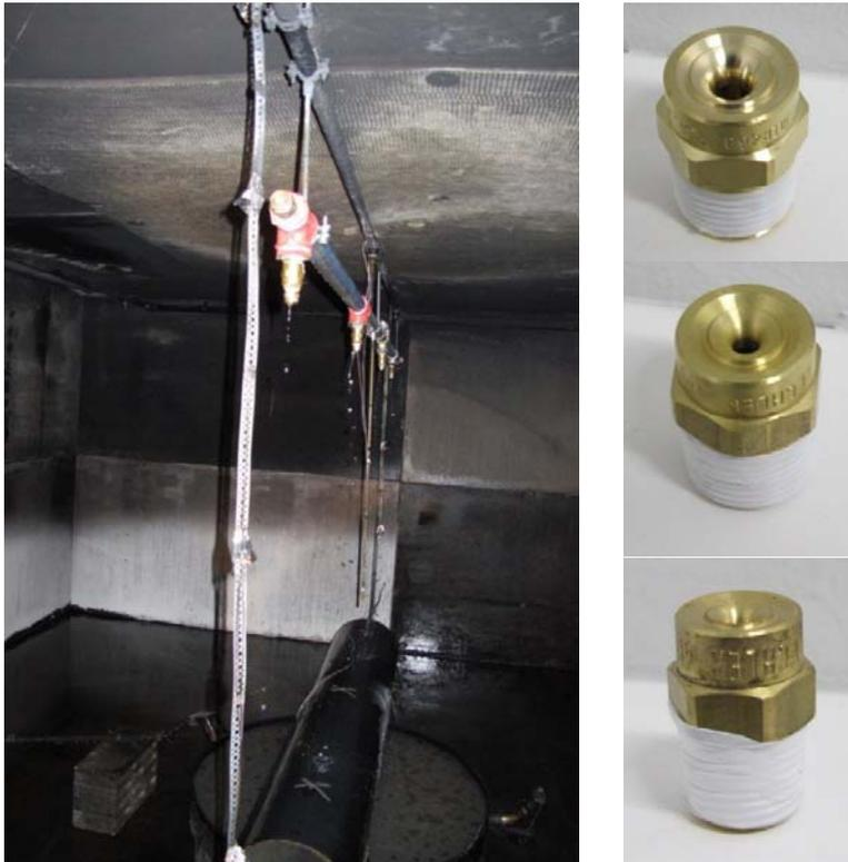
Figure 6 Drencher system and LECHLER nozzles 460.928, 460.728 and 460.608 from top to bottom.
