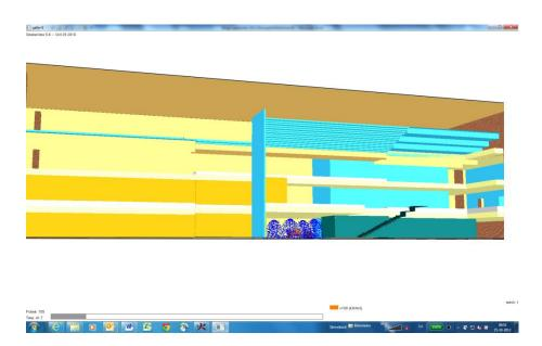
The fire spread over the angle (< 135°) will not occur because the radiation is only 1,8 – 2,1kW/m²
