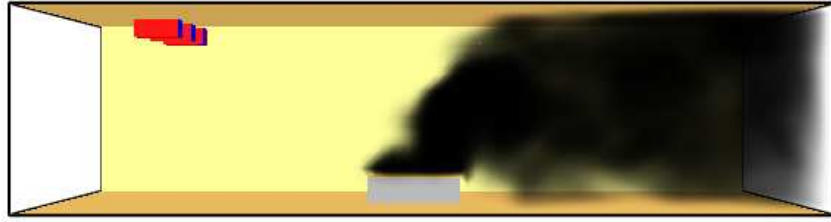
Figure 8: Smoke development with water mist system
