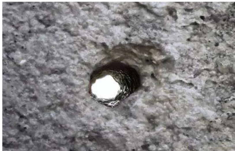
210mm concrete block pierced in 47 secs.
