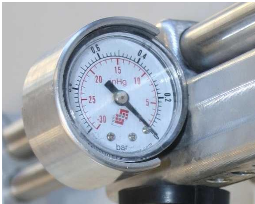
Vacuum meter fitted on the lance 0,5 - 0,6 bar with thin walls 0,2 bar with thick walls
