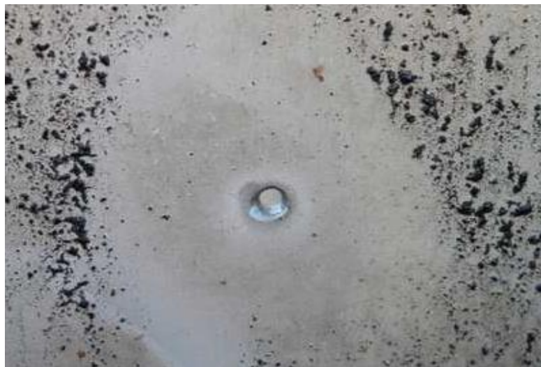
5mm steel sheet pierced in 14 secs. 10mm steel sheet pierced in 31 secs.
