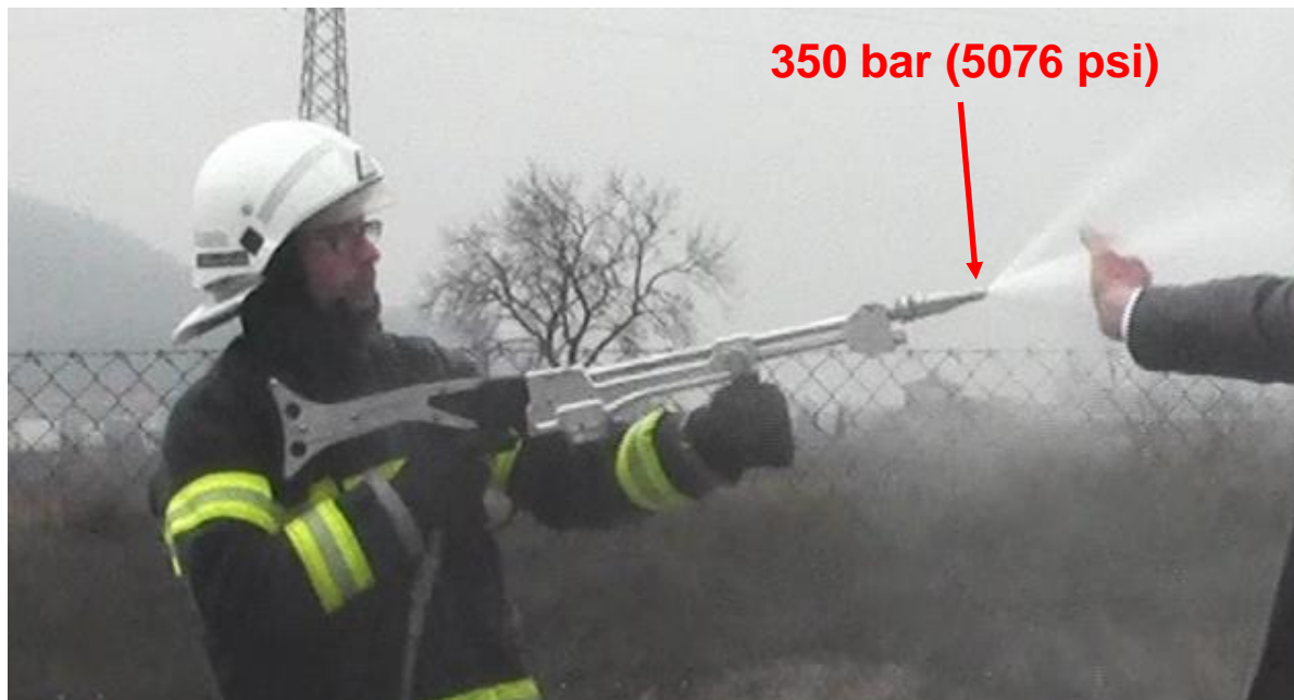
Safety with Water Mist nozzle @ 30 cm (11,81 in)
