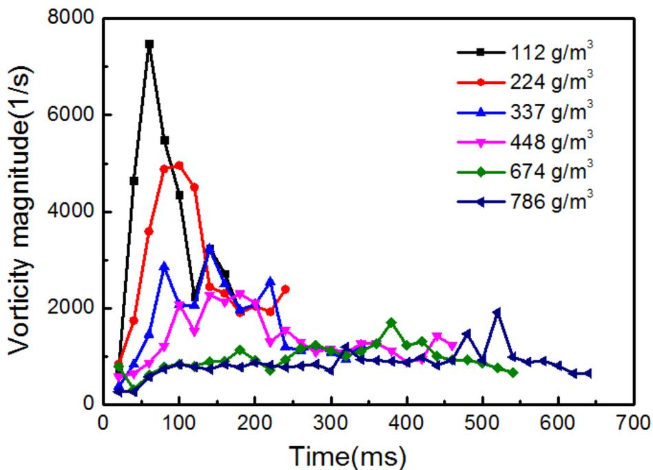
Figure 20 Effect of spraying concentration on vorticity magnitude
