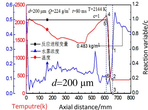
Figure 11 Effect of water mist diameter to contact degree between water mist and flame front
