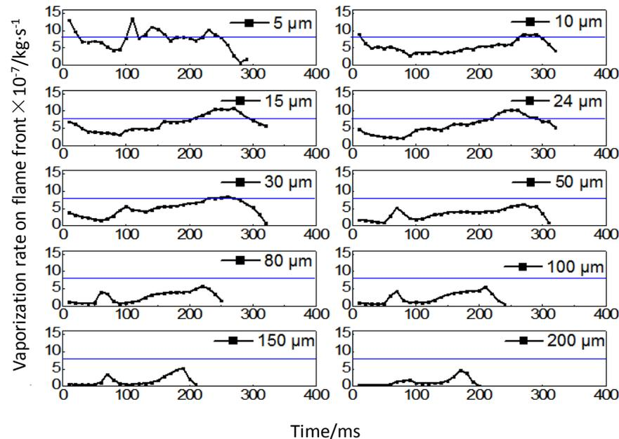
Figure 13 Effect of water mist diameter to the vaporization rate of water mist ( $c=0.01$ )
