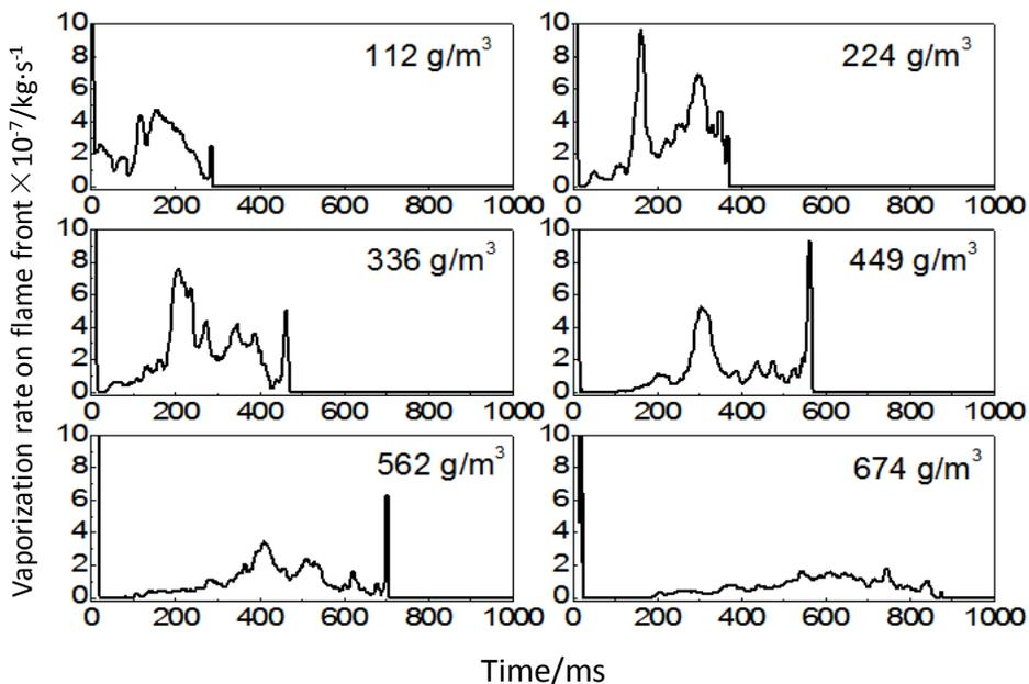
Figure 15 Effect of water mist concentration to the vaporization rate of water mist
