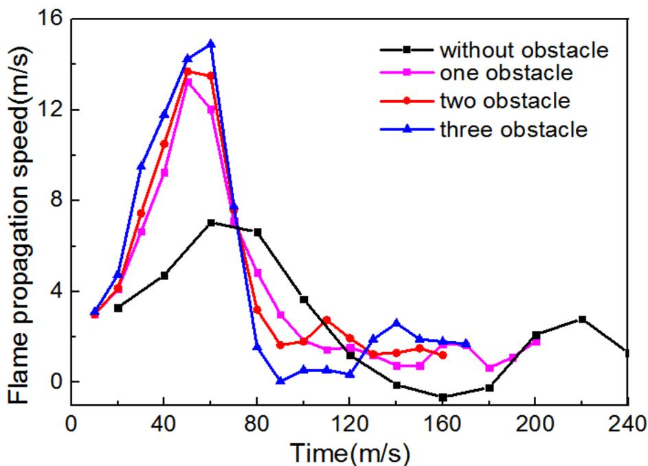
Figure 19 Effect of obstacles on flame propagation speeds
