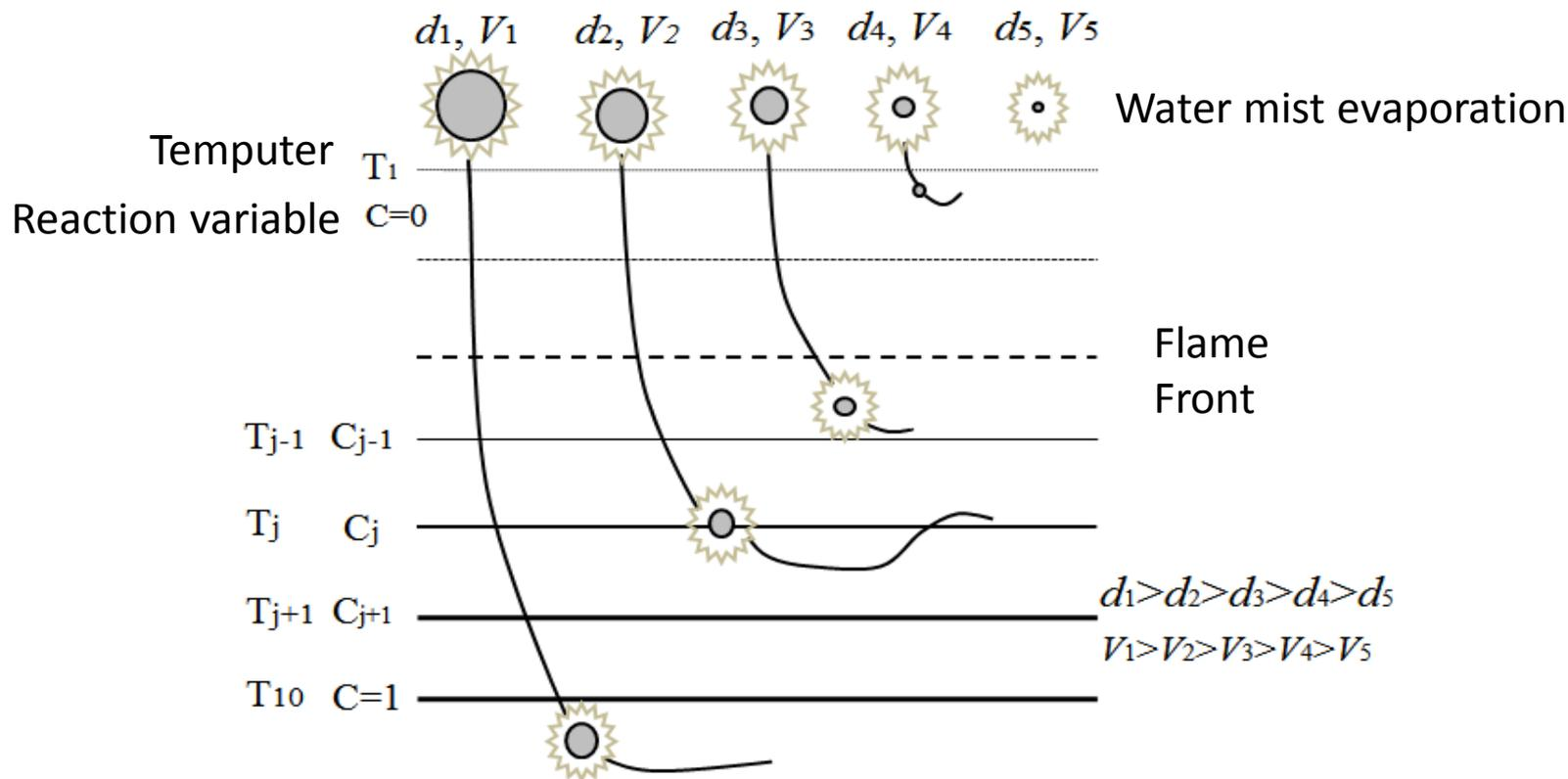
Figure 9 Effect of water mist parameter to contact between water mist and flame front
