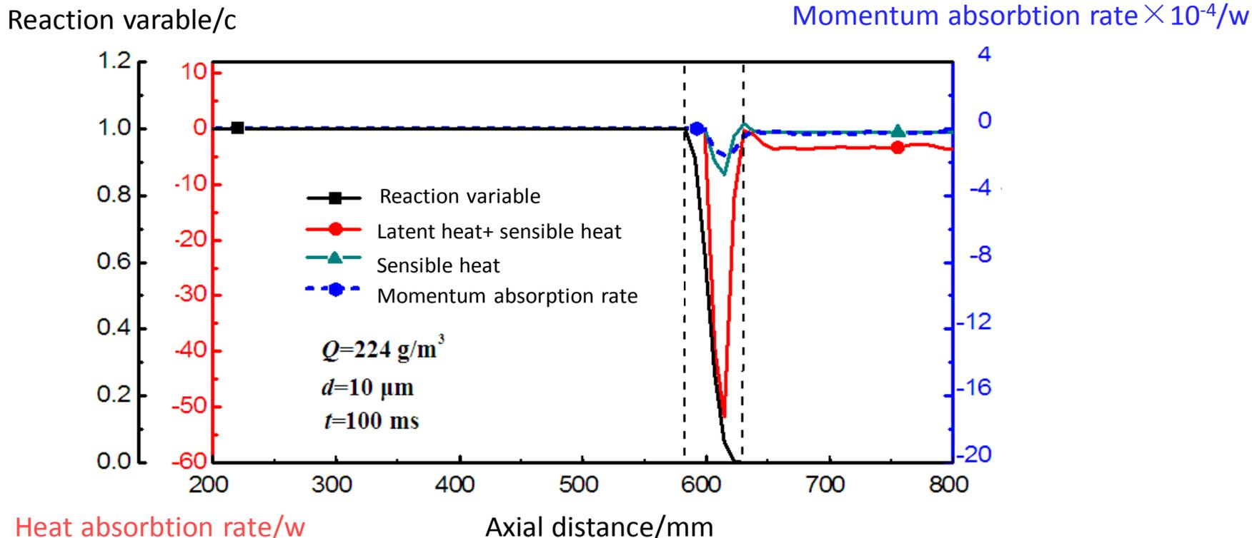
Figure 10 Comparison of energy absorption rate on axial inside vessel
