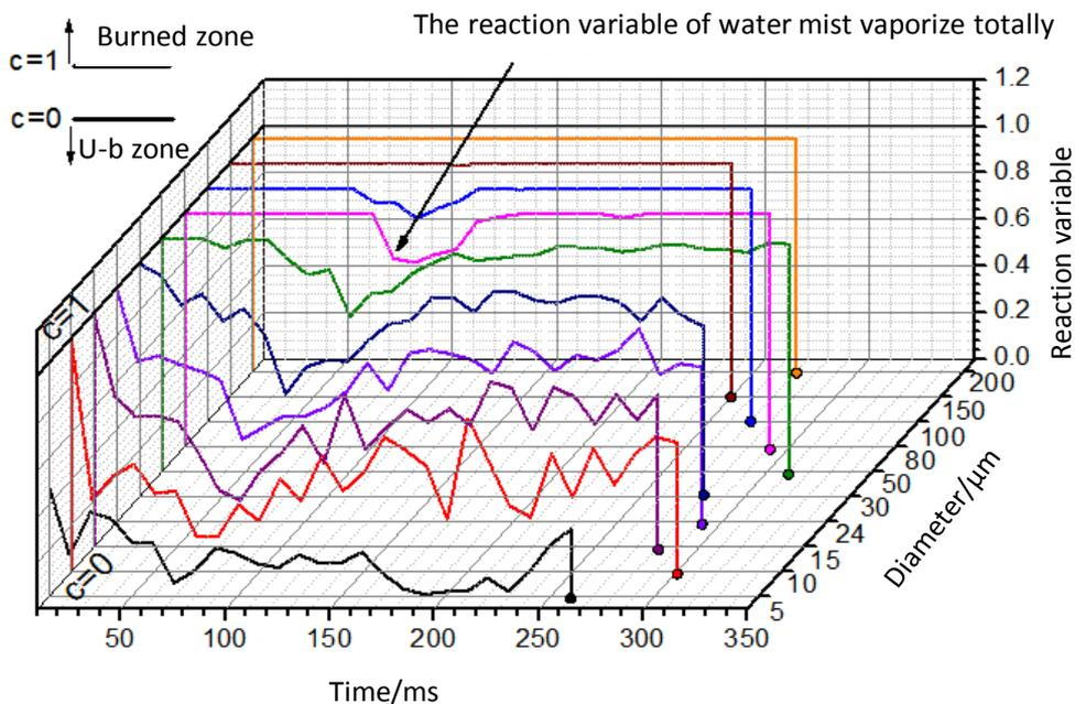
Figure 12 Effect of water mist diameter to the extent of the flame arriving at reaction zone
