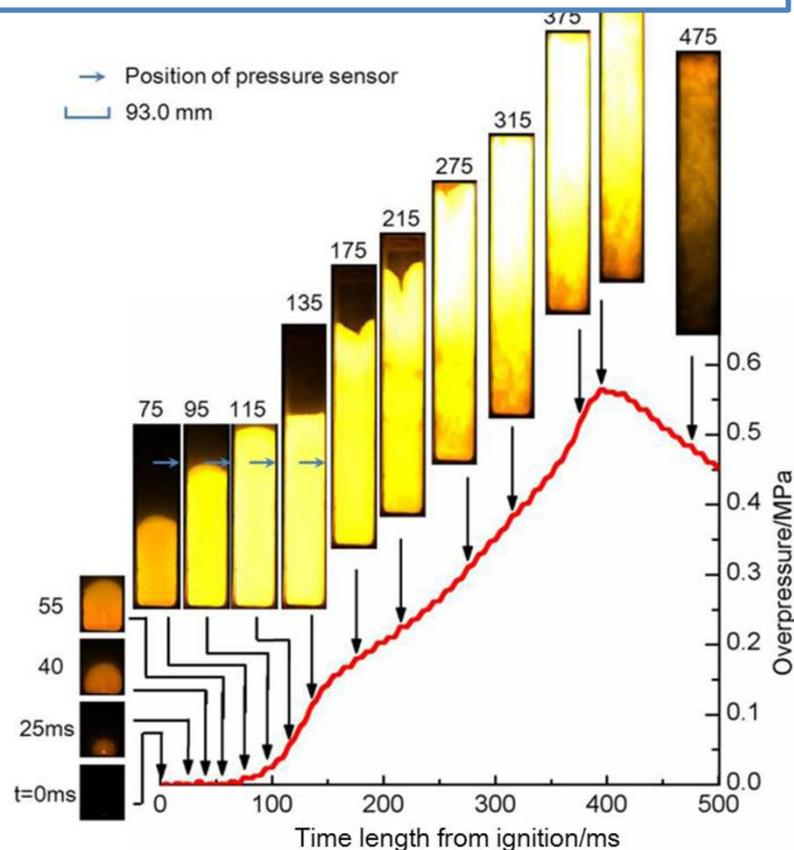
Figure 3 The relationship of explosion overpressure and flame propagation
