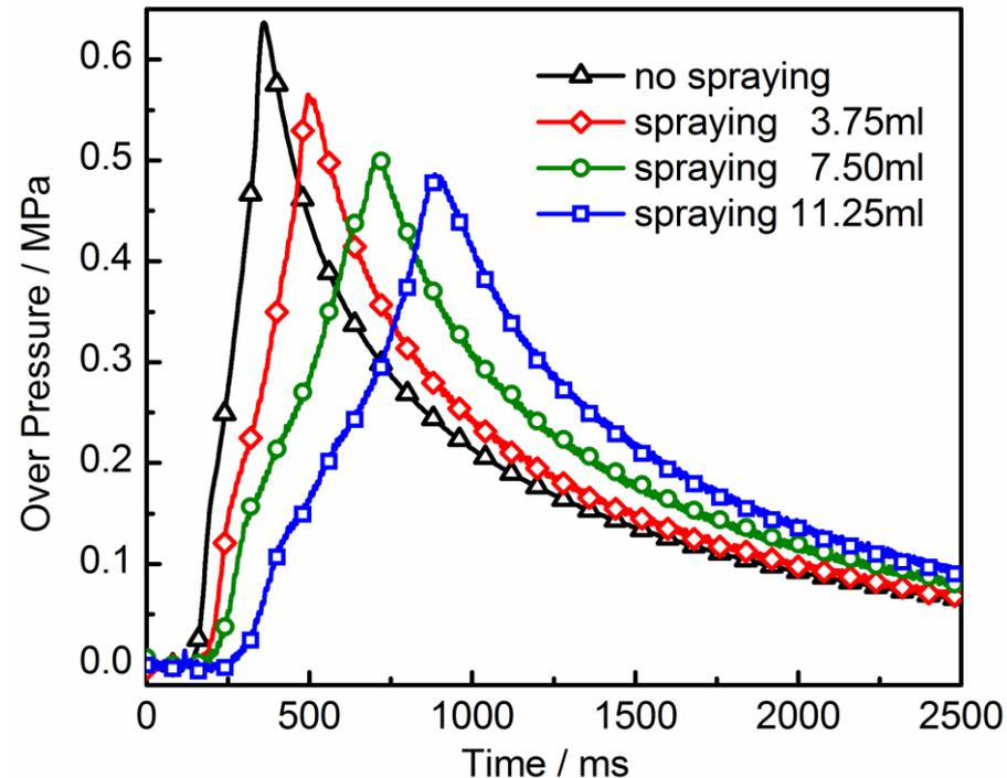
Figure 2 The Pressure histories under different spraying conditions
