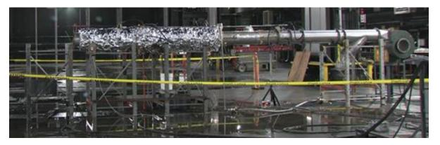
Duct insulated to simulate the thermal response of 0.3-m diameter combustible ducts made of:
