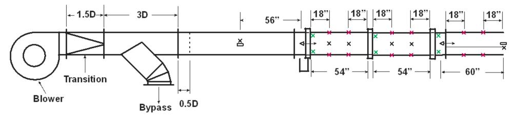
× TC for gas temperature in duct centerline, K-type, 26 gage
