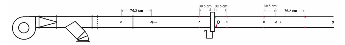
imes TCs in the duct centerline, K-type, 26 gage
