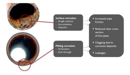
Corrosion is no more present in water mist systems than in sprinkler systems but, due to the smaller orifices present in water mist nozzles, the products of corrosion could impair a water mist system
