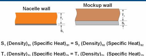
$\Gamma_1$  (Density)<sub>T1</sub> (Specific Heat)<sub>T1</sub> –  $\Gamma_2$  (Density)<sub>T2</sub> (Specific Heat)<sub>T2</sub>
