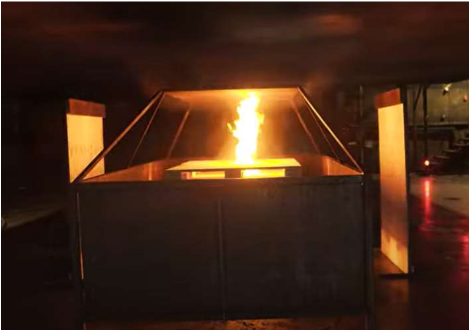
Fig. 12 Example of MSC.1/Circular.1430 mock-up, 2,5 [m] ceiling height
