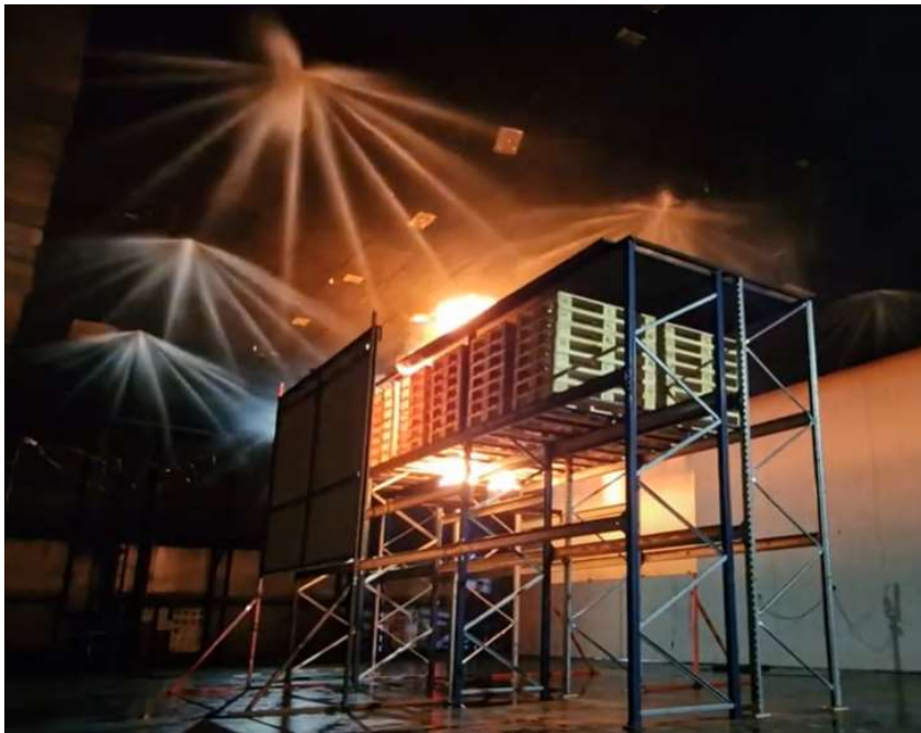
Fig. 14 Example of MSC.1/Circular.1430 mock-up, 5 [m] ceiling height – fire test
