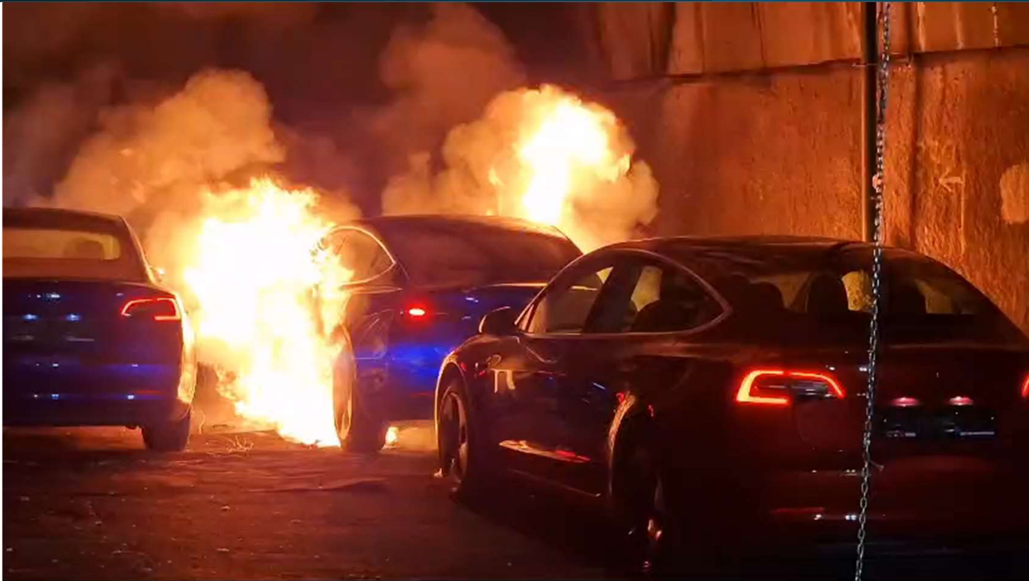
Fig. 9 Example of fire spread, brand new EV fire in underground structure, laboratory conditions – tunnel. Acknowledgments to Reliable Sprinklers Inc. 14
