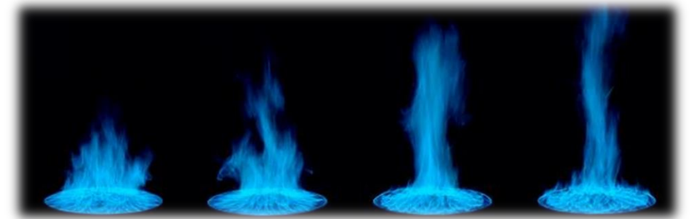
Instantaneous digital images 132 ms apart in the pulsing 1 m diameter methanol pool fire [Sung et al., 2021]
