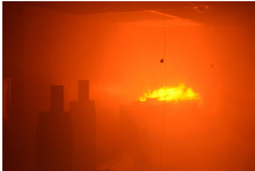
Figure 9: Cooking oil fire with nozzle at 1.5m distance test in progress
