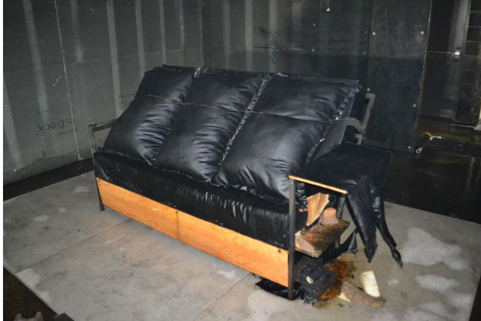
Figure 8: Couch fire load at the end of test with load on centre of room
