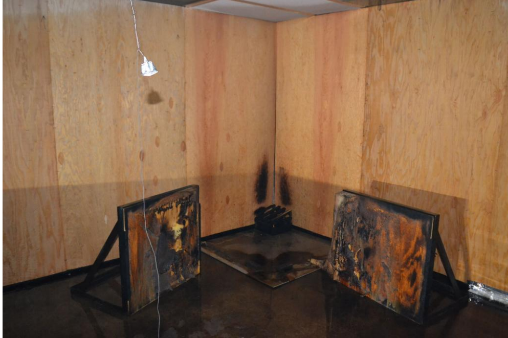
Figure 6: Corner test fire load at the end of fire test (with obstruction)
