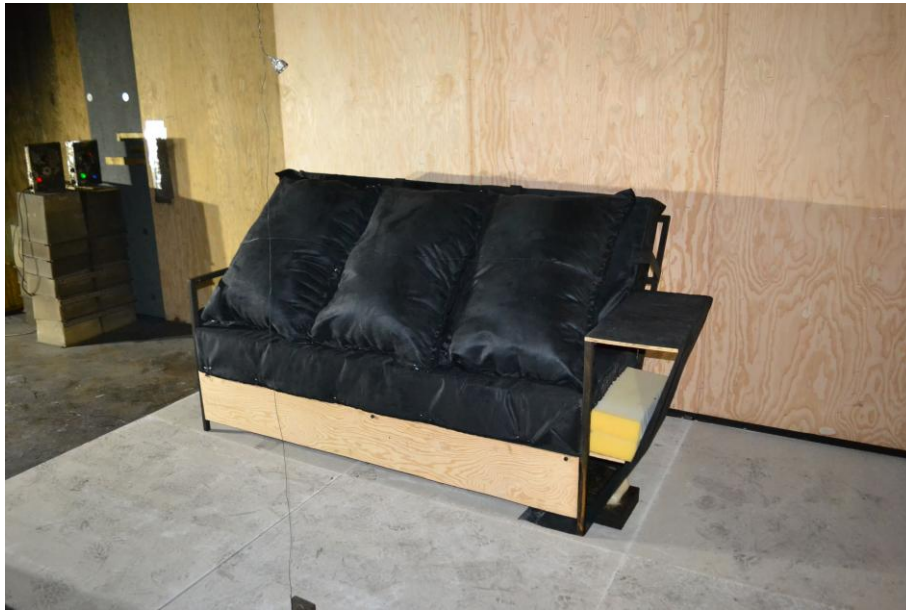
Figure 5: Custom developed couch for UL 2167A, the "couch from hell"
