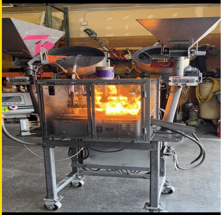
APPLICATION OF WATER MIST FIRE SUPPRESSION FOR AMMUNITION LOADING MACHINES
