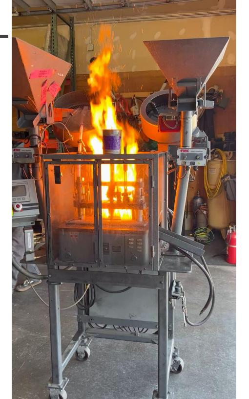
APPLICATION OF WATER MIST FIRE SUPPRESSION FOR AMMUNITION LOADING MACHINES
