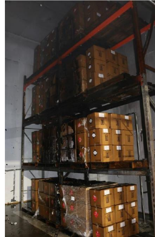
Main fuel array, 4-tiers 28 containers breached
