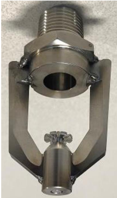
Nozzle (prototype) 150 \mu\text{m} at 60 bar 34 liter/min Stokes number: 1.2
