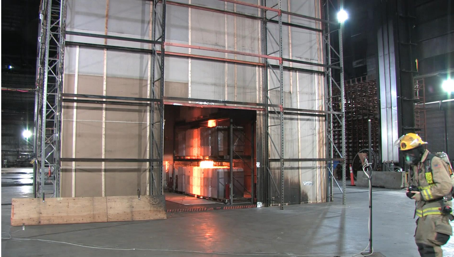
4-tiers rack storage, uncartoned 19-L containers (video 2:00 after ignition)
