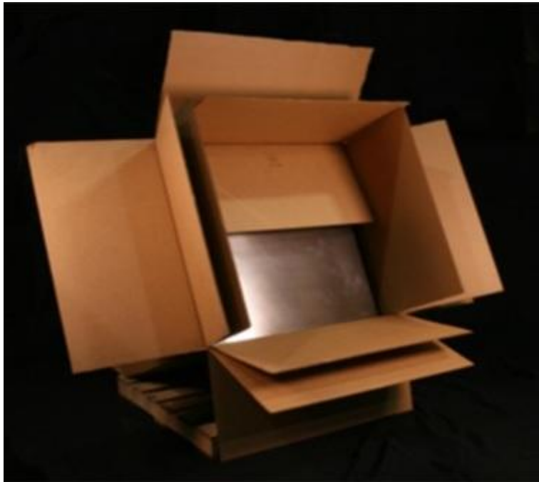
FM HC-2 Fire Hazard
