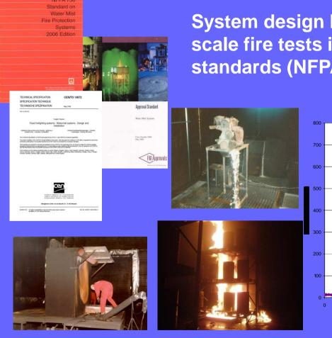
System design based on application related full scale fire tests in accordance to water mist standards (NFPA 750, FM 5560, EN TS 14972)
