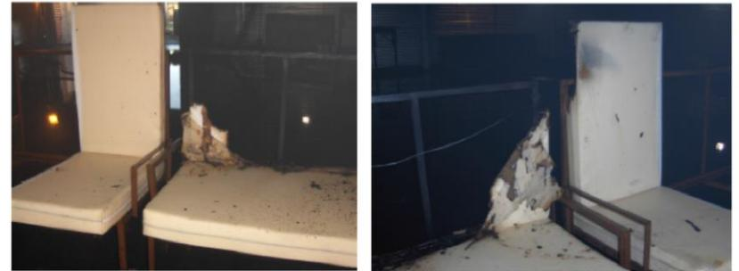
94% damage on backrest on centre sofa, the fire jumped to the right target sofa, this resulted in 1% damage on the backrest. Seat mattress had 3% damage.
