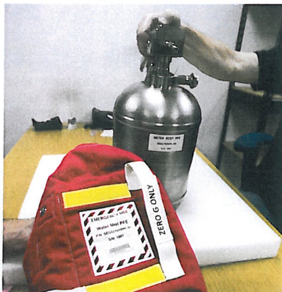
Portable water mist fire extinguisher flight unit at NASA Johnson Space Centre.
