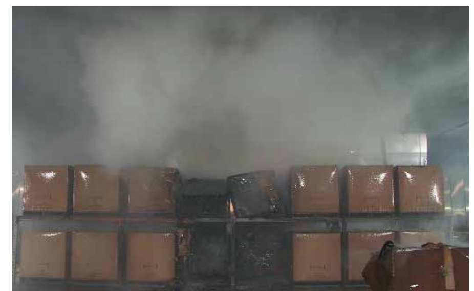
▲ Fig. 2 - Fire test of automatic water mist nozzles over cardboard boxes conducted under the moveable ceiling in the Large Burn Laboratory at the FM Global Research Campus in Glocester, Rhode Island, USA. As the fire grows, it triggers multiple water mist nozzles. The fine droplets are sucked into the base of the fire and flash to steam, depriving the fire of essential oxygen.
