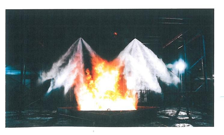
diversity of water mist because due to the small droplets we have a suppressant agent that is applicable on a broad range of fire types.
