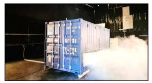
Water mist has proven to be highly effective against emerging risks, such as lithium-ion batteries and battery energy storage systems (BESS). As a highly efficient coolant, it requires only a limited amount of water and does not rely on enclosures to operate, unlike many other technologies. Additionally, water mist is eco-friendly, utilising only water in its operation. (SUVEREN / IFAB)
