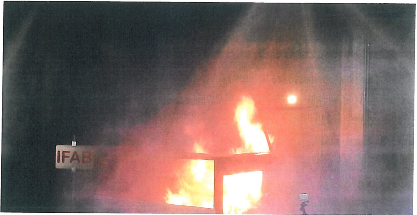
▲ Watermist activation in SUVEREN fire test with electric vehicle.
